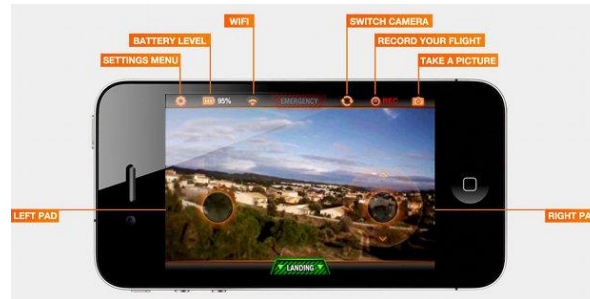
Parrot AR Drone – Smart phone control panel – including live video feed. Images Credit: Parrot Company.
