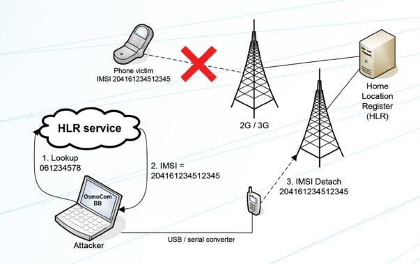
Figure 1 Schematic of an IMSI-detach attack.
