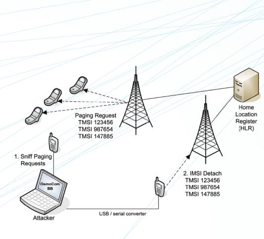
Figure 2 Schematic of a large scale attack.
