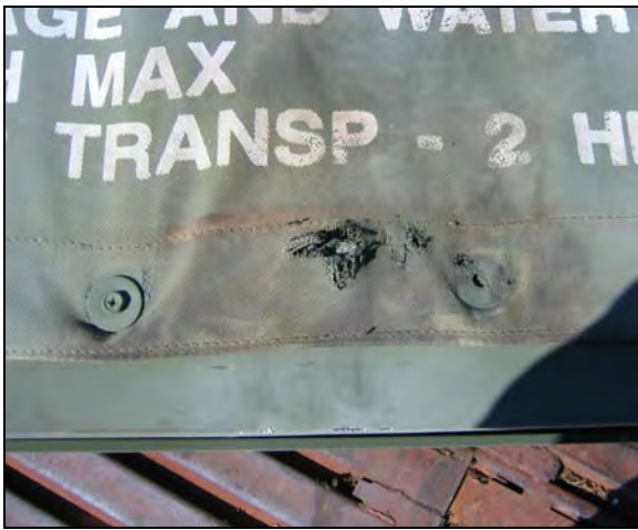
Figure N-8. Example DSL Strike Damage.
