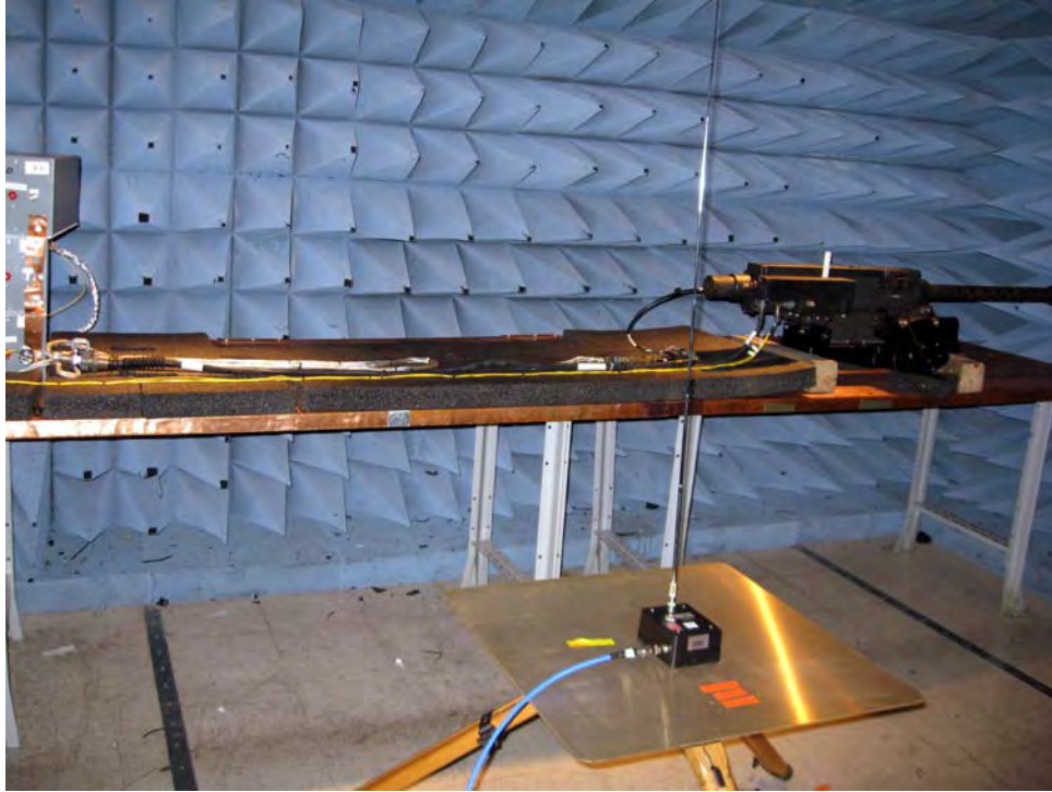
Figure K-6. Sample Emissions Set-up Photo for MIL-STD-461F.
