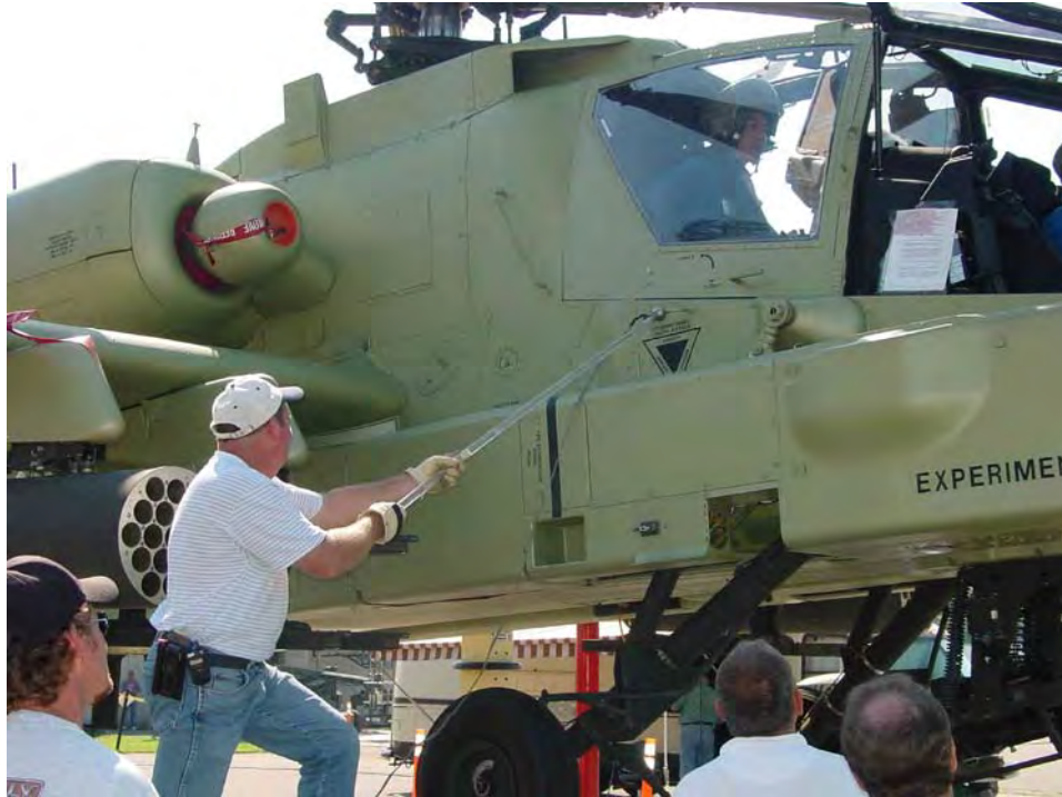
Figure F-6. Example P-Static Test Setup – Discharging the Aircraft.
