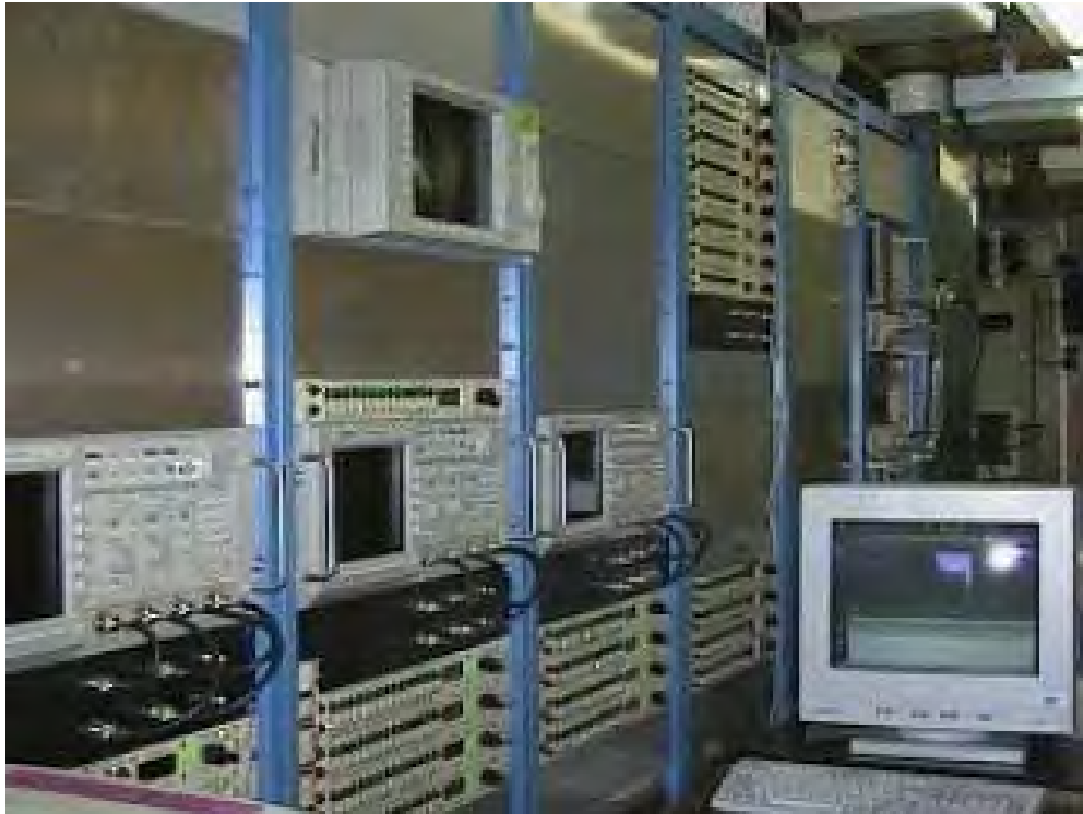
Figure D-2. Typical EMP Instrumentation Set-up.
