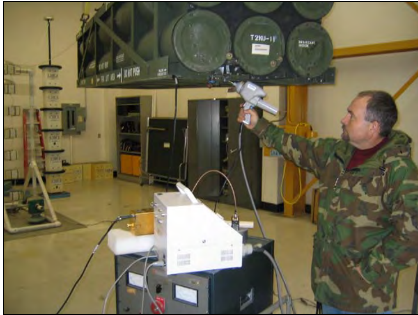
Figure M-3. Typical PESD Test Setup – Sling Loaded.
