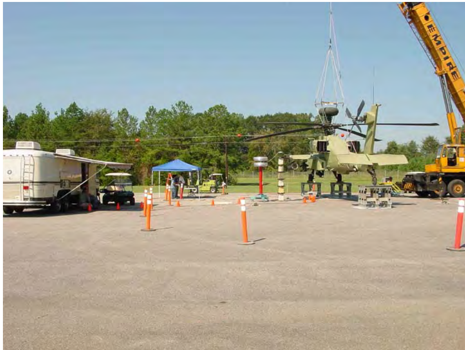
Figure F-3. Example P-Static Test Setup.
