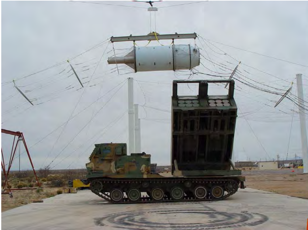
Figure D-1 Typical EMP Test Set-up.
