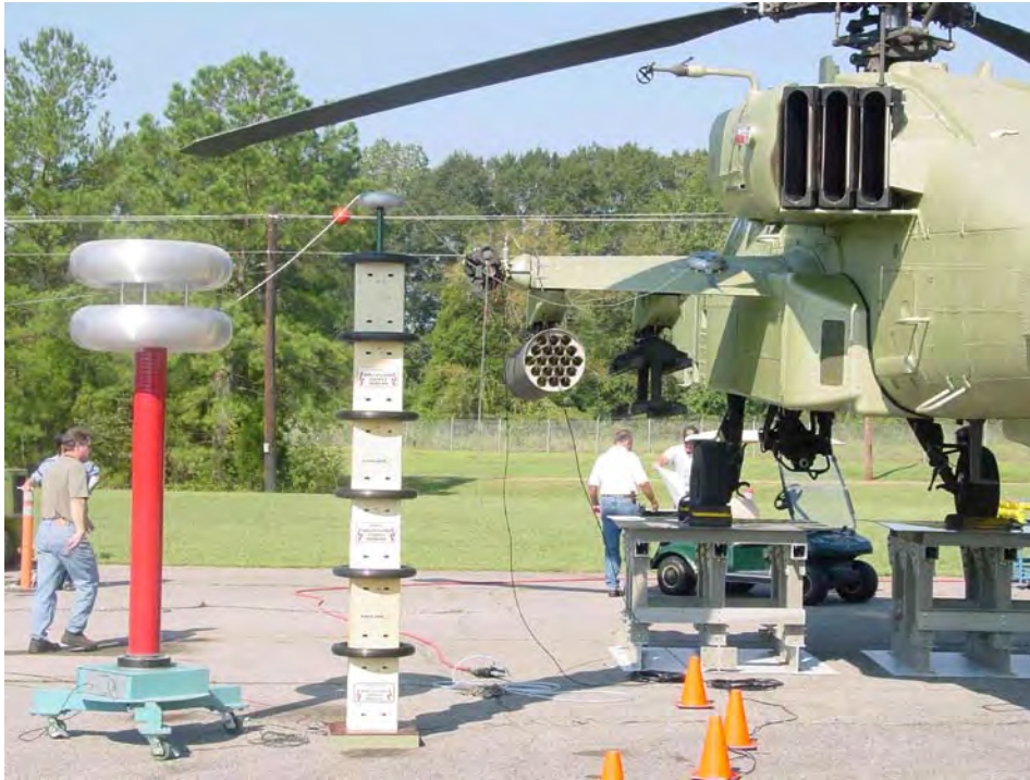
Figure F-4. Example P-Static Test Setup with Charge Generator & Voltage Divider.
