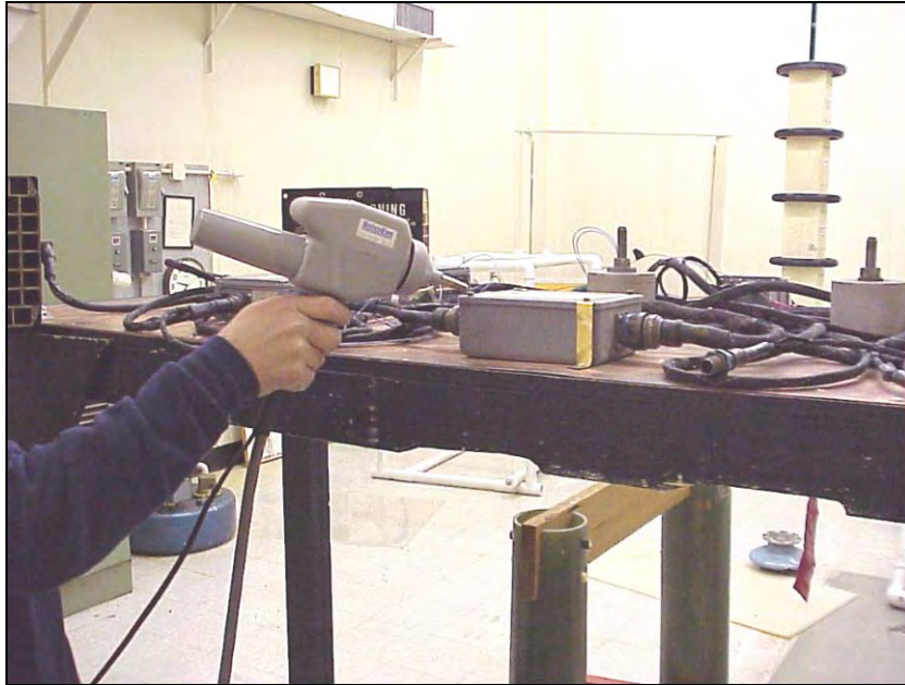
Figure M-2. Typical PESD Test Setup Component Level.
