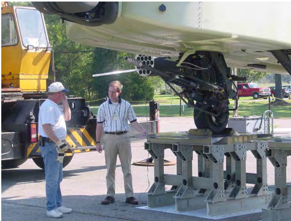
Figure F-5. Example P-Static Test Setup – Isolation Test Stand Close-up.
