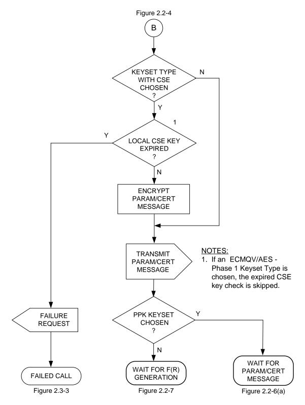
Figure 2.2-5 Parameters/Certificate Message Transmission
