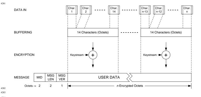
Figure 3.4-1 Secure RT Asynchronous Data Message Preparation
