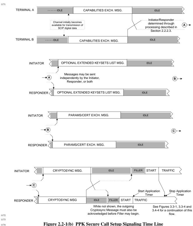
**Editor's Note:** Note that the dotted lines indicate a functional relationship where one message must be received before the second message can be formatted and transmitted.
