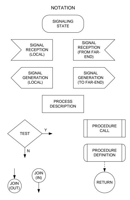
**Figure 1.7-1 Process Diagram Symbols**
