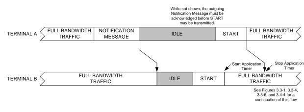
Figure 2.3-1(c) Notification Message Signaling Time Line (Full Bandwidth to Full Bandwidth)
