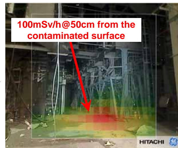
Image acquired at the large carry-in entrance after BG correction (Angle of elevation: 10 degrees)
