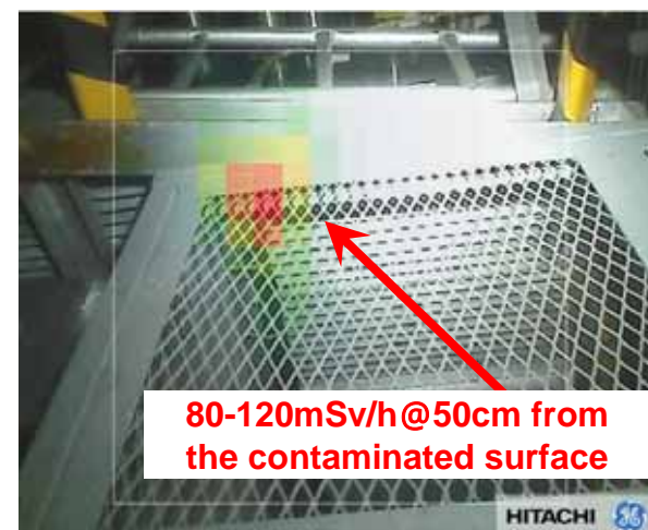
Image acquired at south side aisle after BG correction (Angle of elevation: 50 degree)
