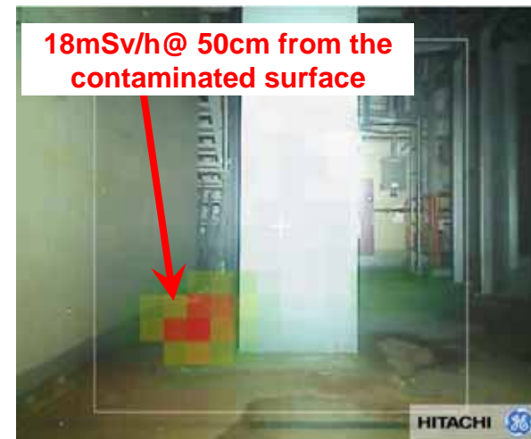
Image acquired at north side aisle after BG correction (Angle of elevation: 0 degree)
