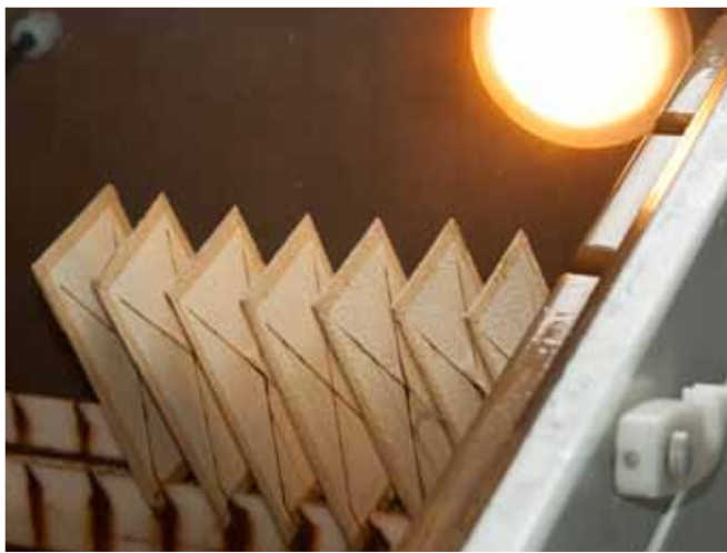
The salt Test. Milspec paint samples requires 500 hours in this device. Varcol is proven to over 1000.
