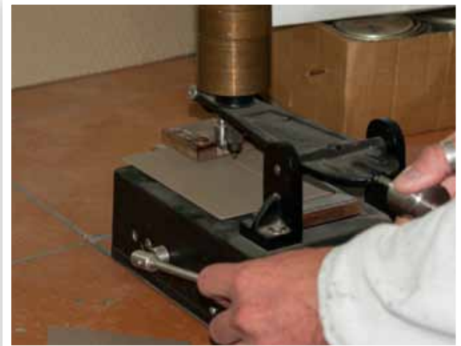
Paint scratch test. Sample paint must not flake off when scratched.
