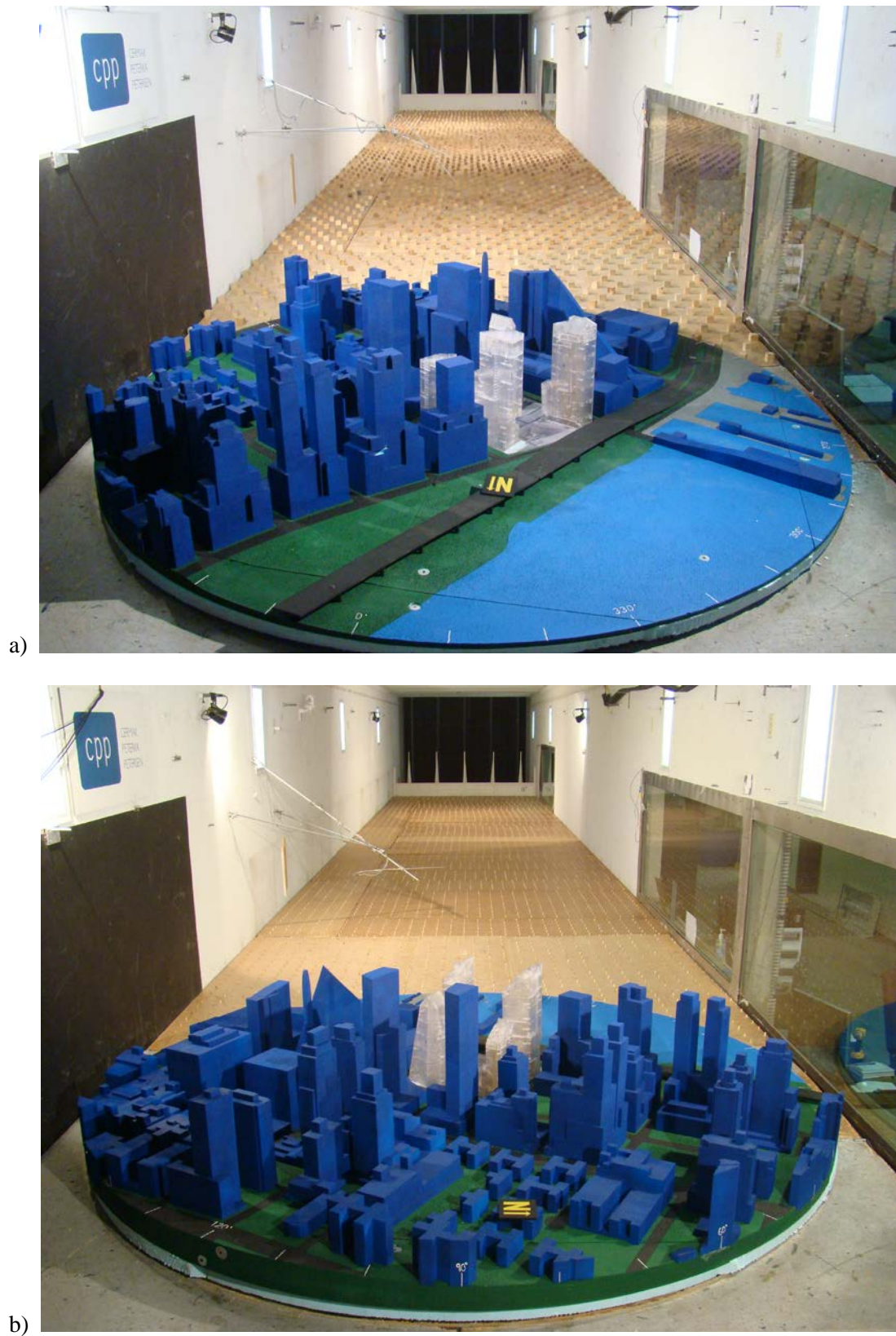
Figure 1. Photographs of the completed model in the wind tunnel: (a) View from northwest, simulating southeasterly wind; (b) View from east, simulating westerly wind. Note spires and trip at entrance to test section, and roughness elements on approach fetch to develop a turbulent boundary-layer flow.
