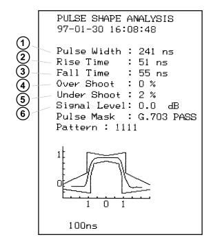
Figure 4 Example of pulse shape measurement screen
