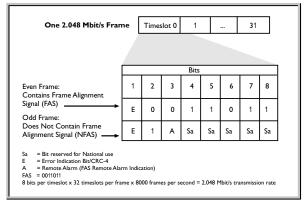
Figure 8 FAS framing format
