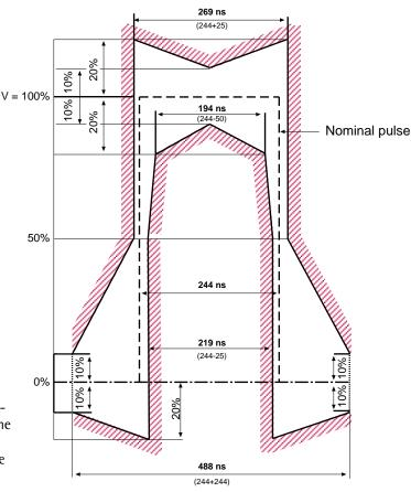
Figure 3 Mask of the pulse at 2.048 Mbps interface
