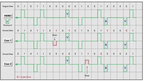
Figure 7 HDB3 error detection
