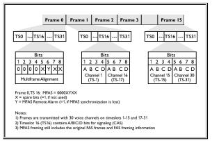
Figure 9 MFAS framing format
