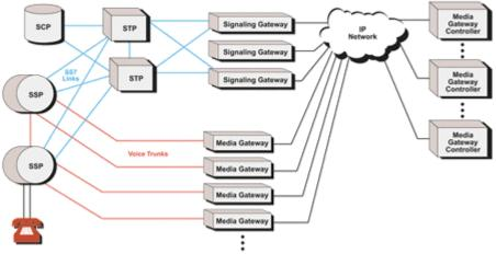
Figure 2. Example of a VoIP network configuration
