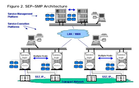
A single instance of the SMP can control multiple IN network elements. All service-deployment and data-provisioning requests are directed to the SMP, which then performs the necessary updates on the IN network element. In addition, the SMP is also responsible for the distribution of data updates across these IN elements.
