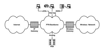
Figure 1. Public telephone network schematic.
