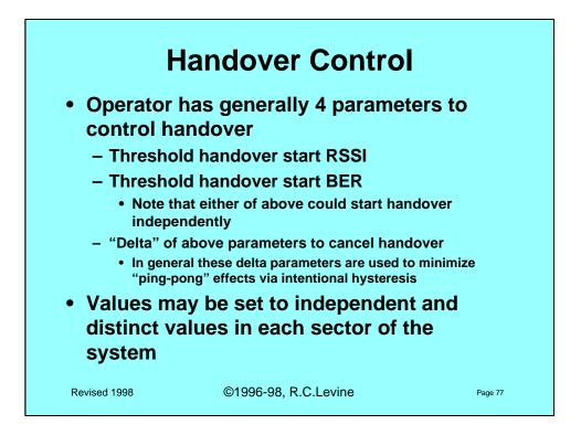
Setting these handover thresholds is one of the few parameters which the operator (as opposed to the manufacturer of the base system) has under control. A lot of experimentation is used to "fine tune" the value of each threshold in each cell or sector.
