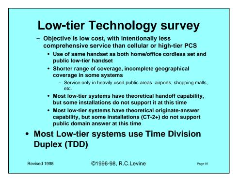
Low tier systems are generally designed to provide limited coverage for a high geographical user and traffic density at lower cost than public domain or high tier cellular or PCS systems.
