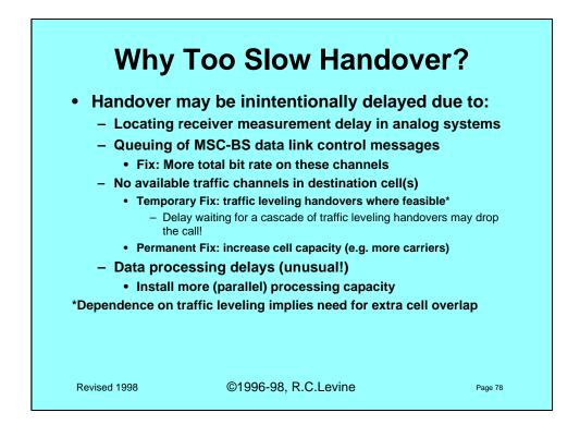
In most cases, although analog cellular systems suffer from problems arising from handoff delay, a properly provisioned digital cellular system should not have any unexpected delays in performing a handoff.
