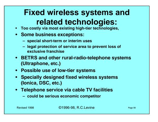
Many other technologies have been proposed for general public PCS use. Some involve radio, others are alternative methods of wire transmission. Most of the radio systems based on cellular or other higher cost technology cannot compete reasonably with ordinary wire landline telephone. Only in special short term applications is high cost wireless useful. It is often installed only to temporarily provide service until replaced permanently by wired telephone service.
