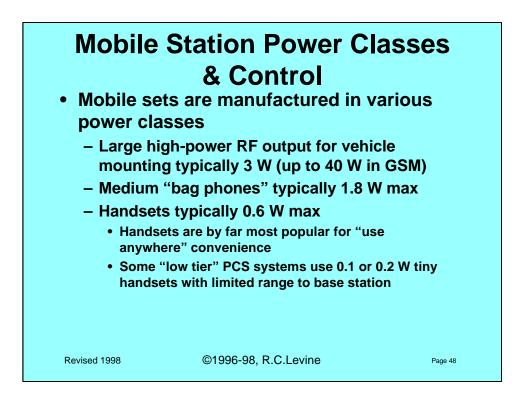
High power class MSs, like the 20 watt vehicle mounted mobile unit in GSM, must have a final PA which can be adjusted for the full range of 16 power steps. They use the lowest power step when they are very close to a base station, or when they are in a small cell.
