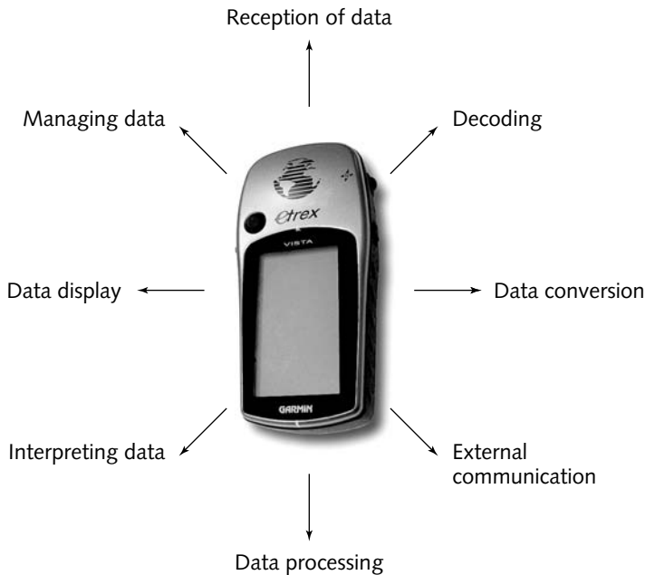
FIGURE 6-1: The basic functions of a GPS receiver
