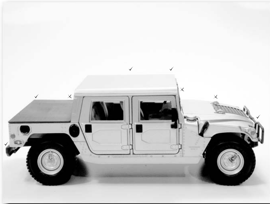
FIGURE 4-10: Good and bad placements for antenna on a car
