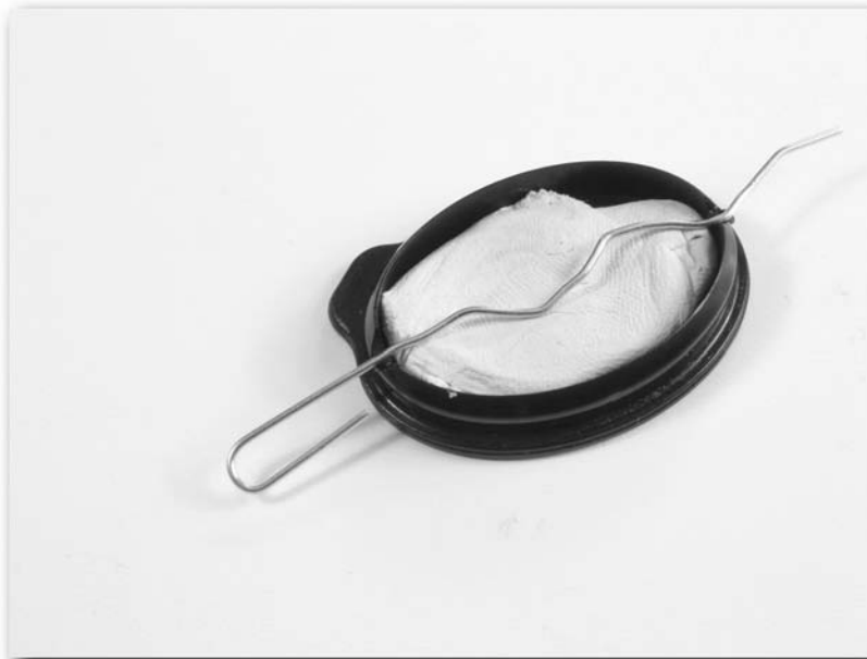
FIGURE 3-17: The top of the completed film pot. Note the notches at either end of the lid accommodating the wire for the terminals.
