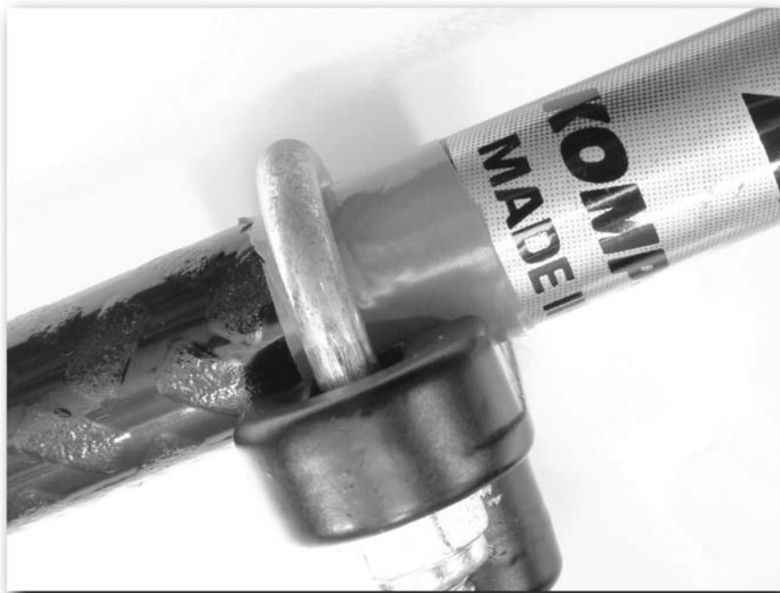
FIGURE 5-35: A layer of tape enables you to tighten the clip without damaging the metal. Even with this protection, however, remember to take it easy when tightening the nuts.
