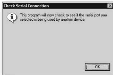
FIGURE 8-16: Testing the connection. This attempts to communicate with the GPS using the connection settings specified.
