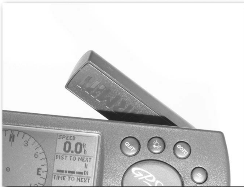
FIGURE 4-4: An antenna at an odd angle is not as effective as one in the vertical position.
