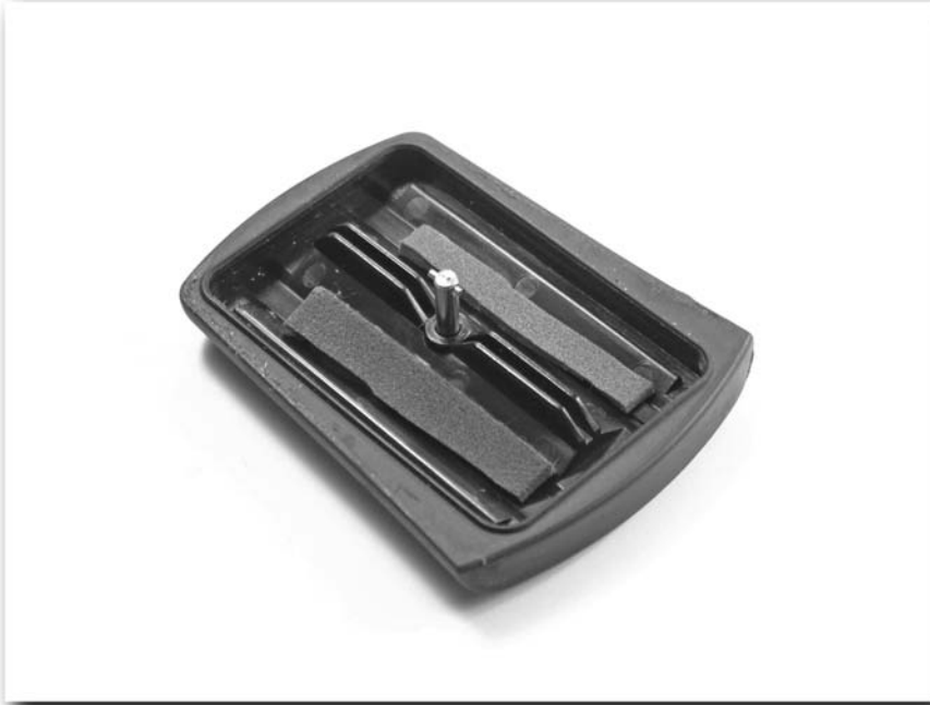
FIGURE 11-34: Pad the battery compartment to prevent power loss.
