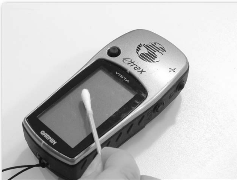
FIGURE 5-3: Carefully clean the screen before applying the screen protector.
