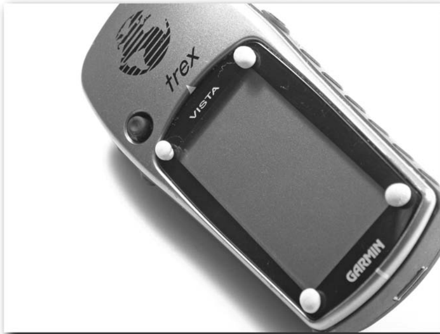
FIGURE 11-33: Rubber bumpers add simple screen protection.
