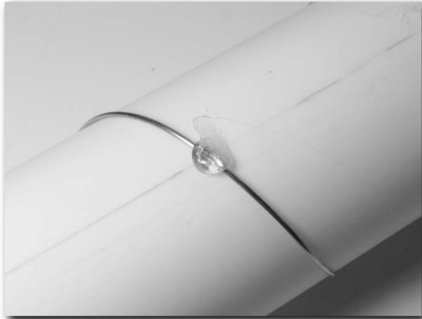
FIGURE 4-19: Partly completed helix coil
