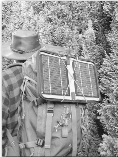
FIGURE 3-22: Solar panel attached to a backpack. This is an ideal way to position such panels when on the move. WILEY.HACKING.GPS.MAR.2005.EBOOK-LING
