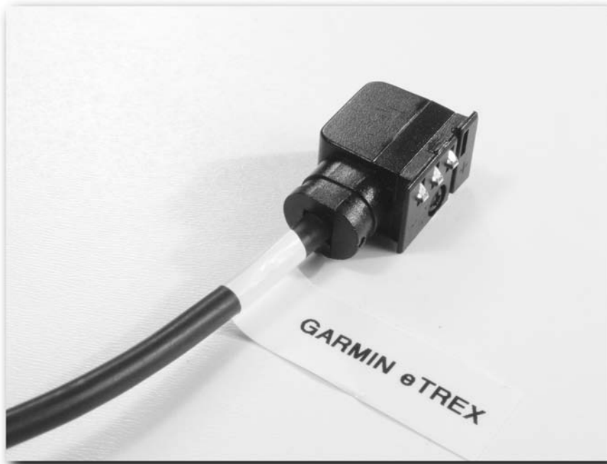
FIGURE 2-23: Label cables clearly to avoid confusion.
