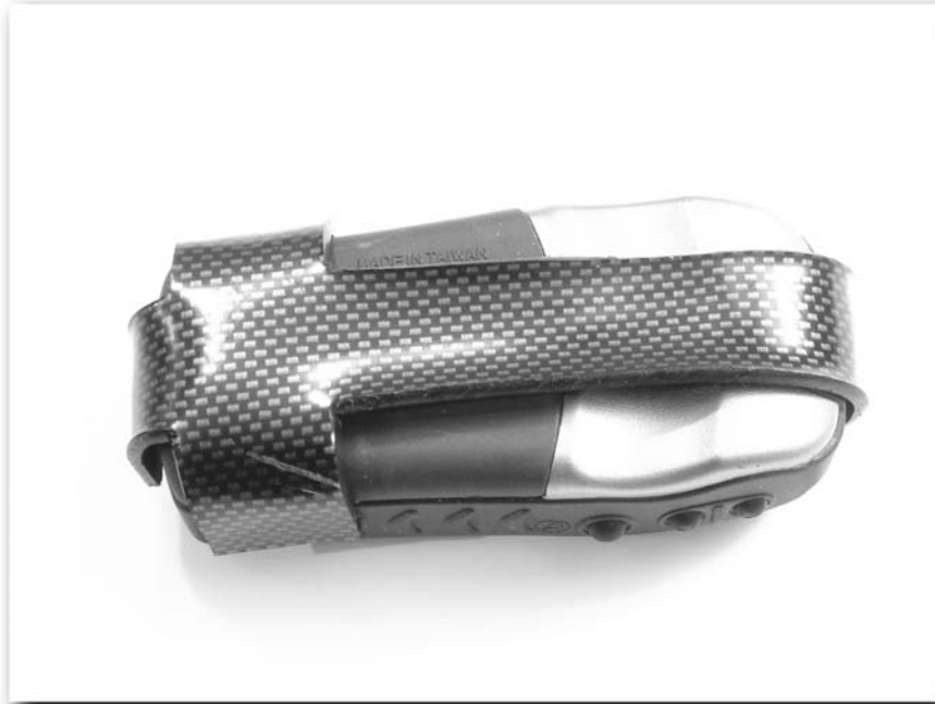
FIGURE 5-40: Mold the warm Concealex on the GPS.
