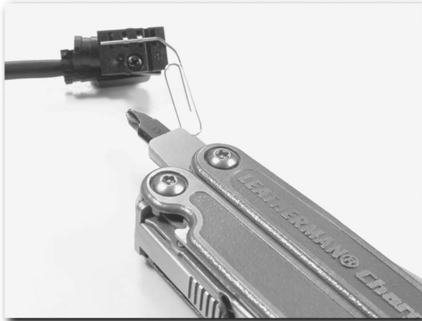
FIGURE 2-14: The single screw holds the connector together.
