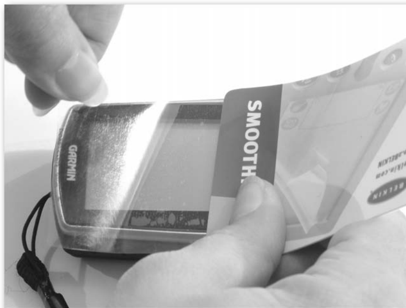
FIGURE 5-6: Using the plastic card to work out bubbles in the plastic film is vital.
