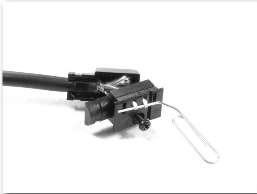
FIGURE 2-13: Use a piece of wire to hold pins in place during assembly.
