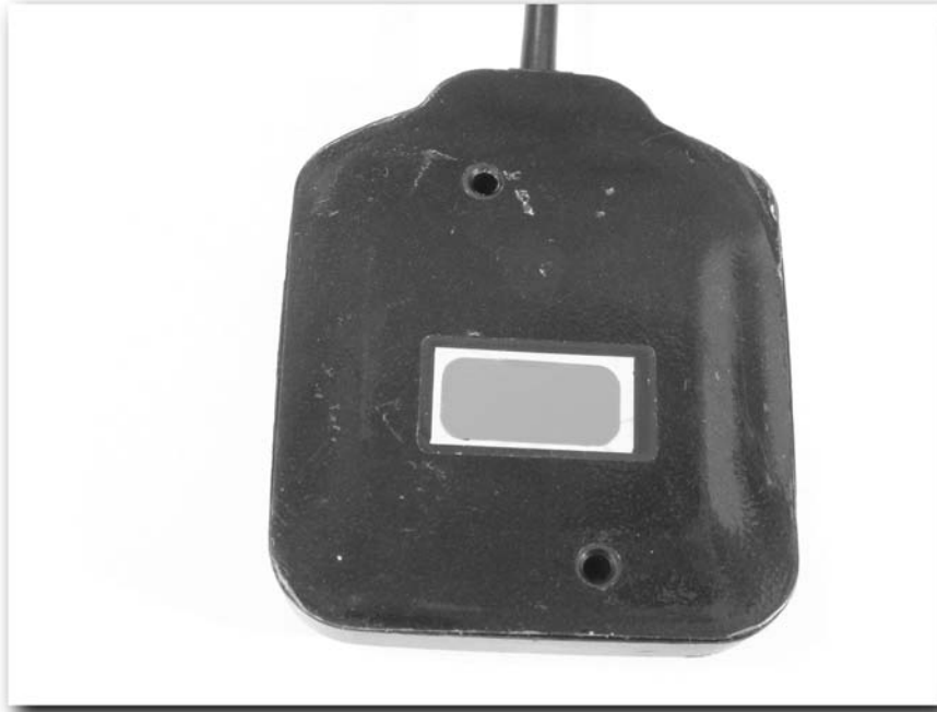
FIGURE 4-8: The external antenna has a strong magnet at the base for affixing to a car roof.
