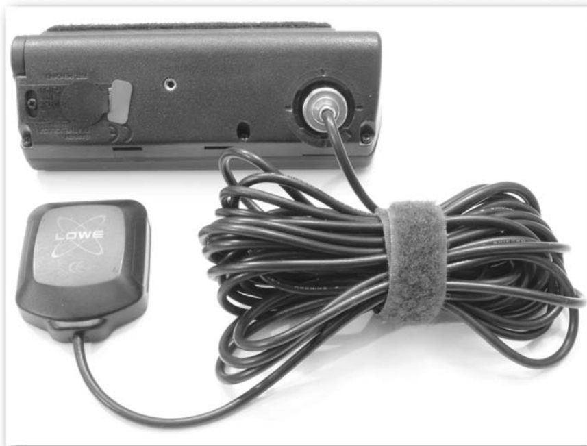
FIGURE 4-7: Lowe external antenna attached to the Garmin III
