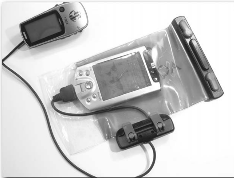
FIGURE 5-24: This Aquapac has a special cable port that enables you to have a cable connected to the iPAQ while in the case.
