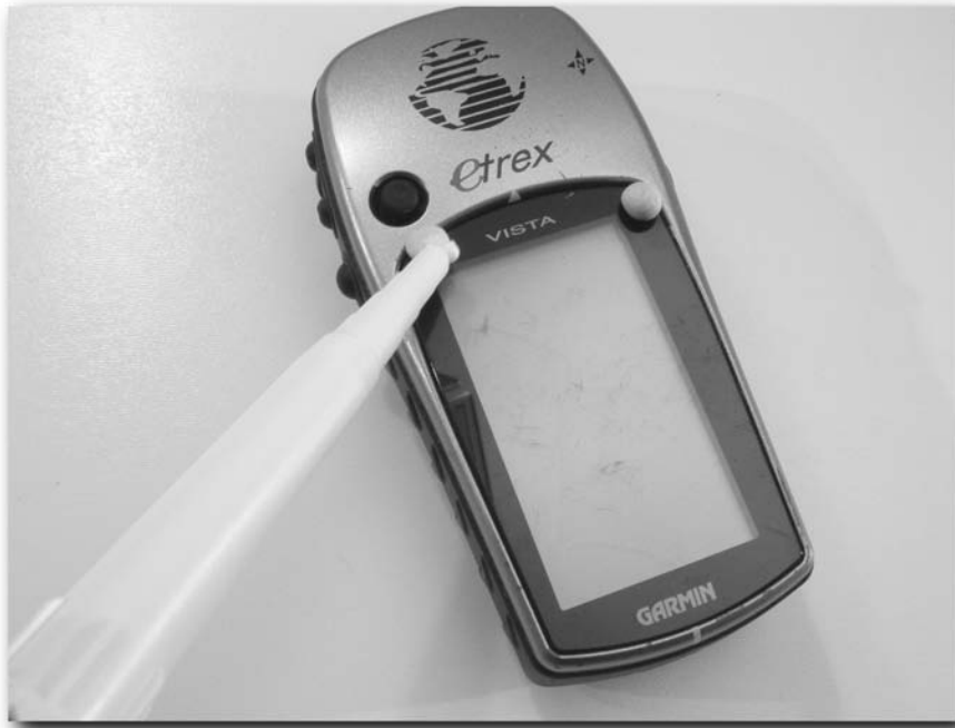
FIGURE 5-9: Apply a few blobs of silicone to the edges of the screen—waiting for it to dry before using.
