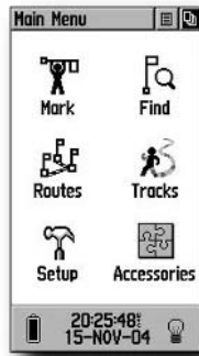
FIGURE 6-2: Healthy battery level on a Garmin eTrex
