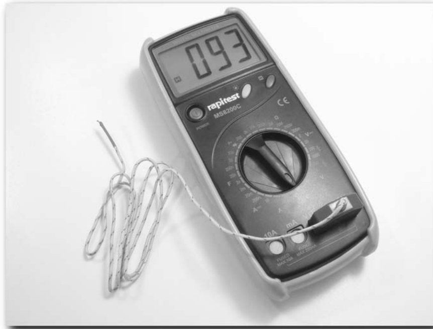
FIGURE 5-37: A multimeter with a temperature probe makes the job much easier.
