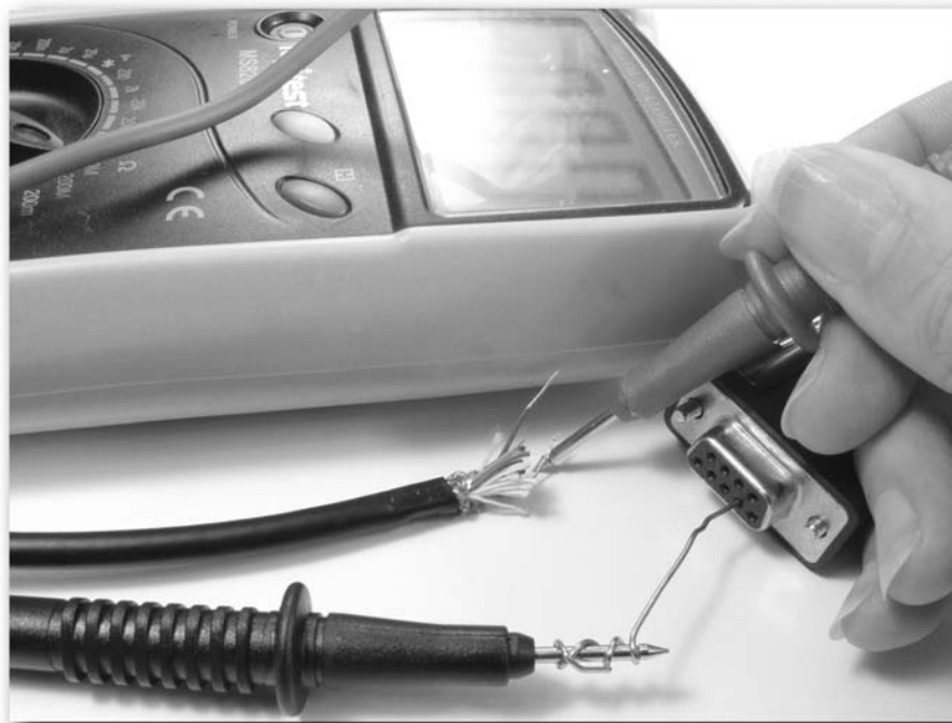
FIGURE 2-7: A multimeter makes it easy to trace what wire goes to which pin.
