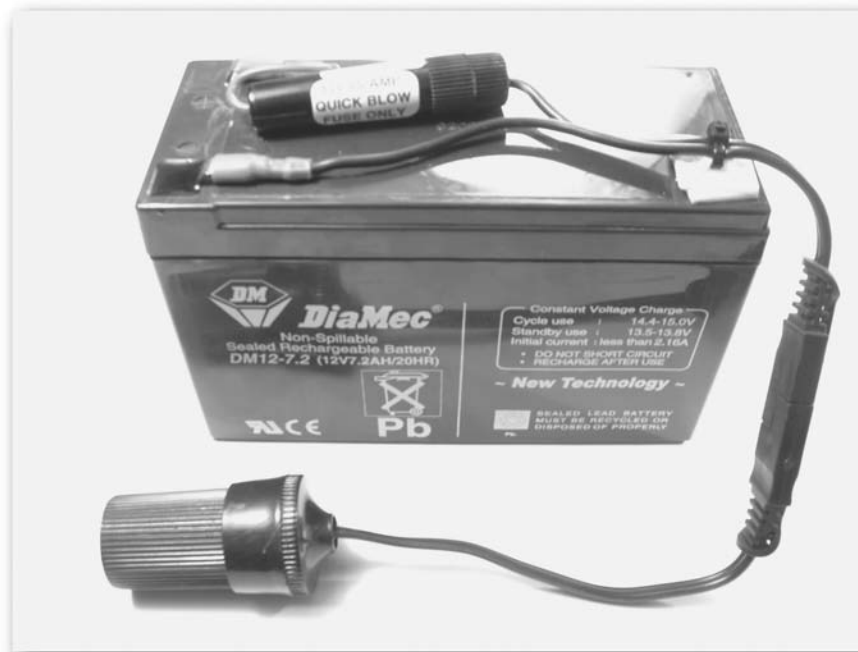
FIGURE 3-5: A fused 12-volt lead-acid battery
