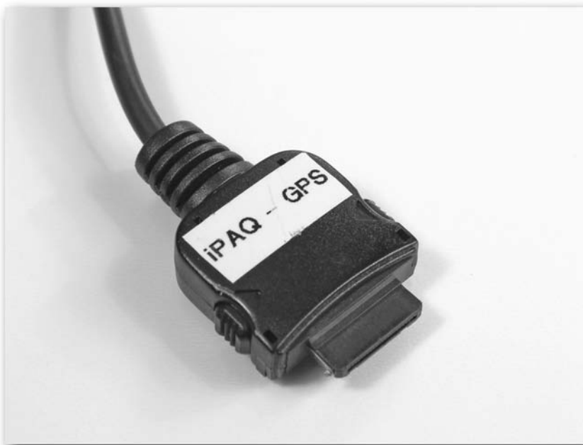
FIGURE 11-17: Clearly labeled cables
