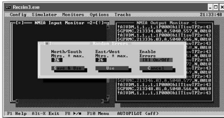
FIGURE 9-11: Adding errors to the simulated GPS data
