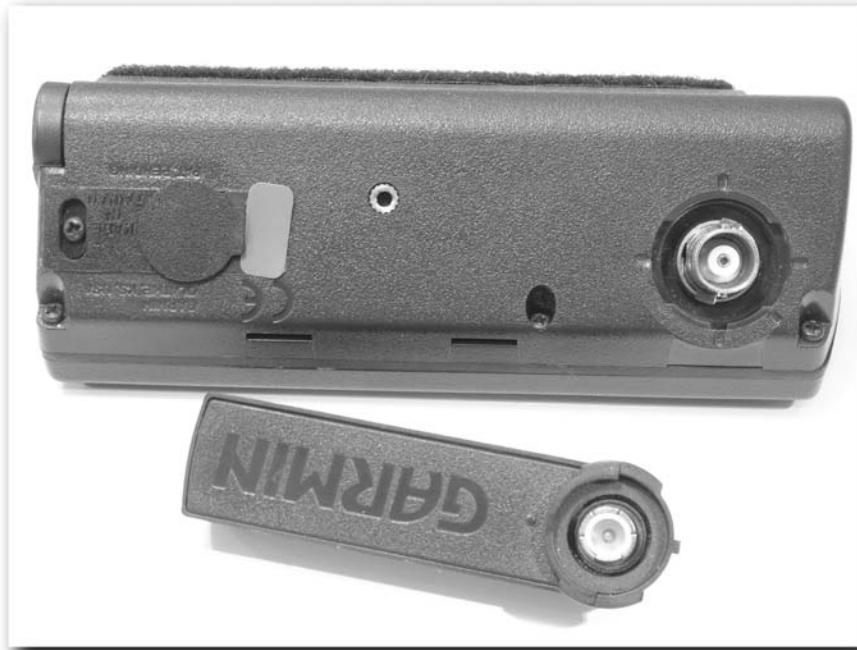
FIGURE 4-6: A Garmin III GPS receiver with the antenna removed
