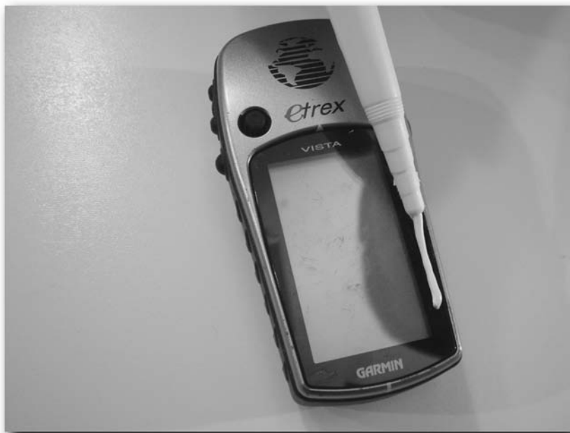
FIGURE 5-10: Ridges offer greater protection against scratches and bumps.
