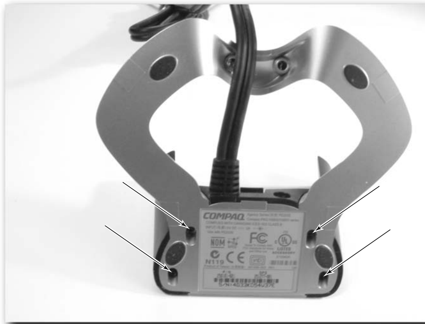
FIGURE 2-25: You need to undo these screws.
