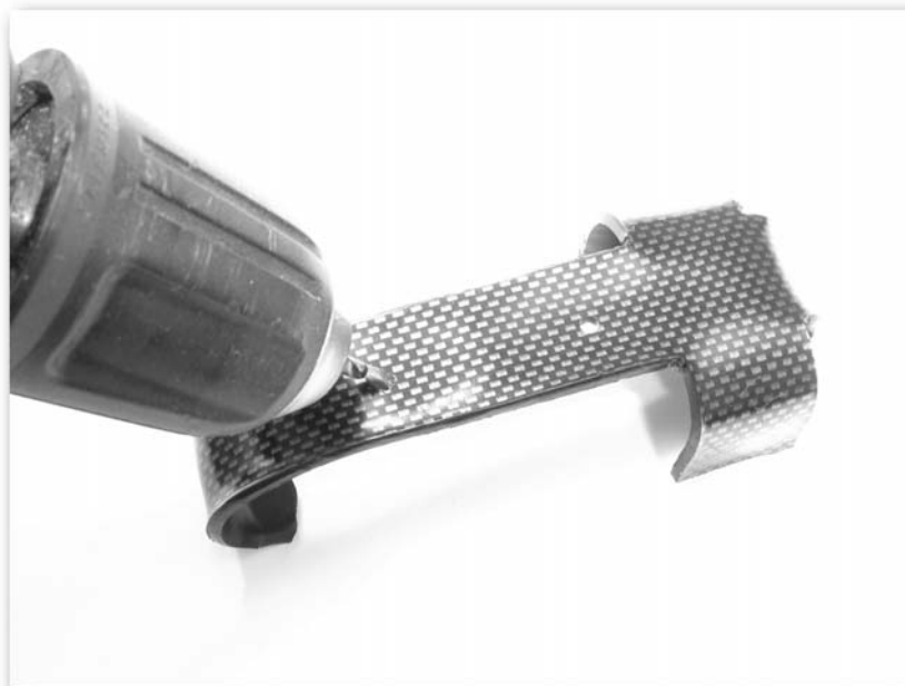
FIGURE 5-45: Drilling the holes to attach the Tek Lok
