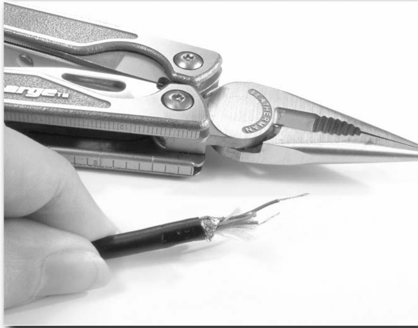
FIGURE 2-8: Trimming back the sheathing
