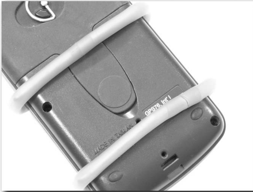
FIGURE 5-16: Overlapped tubing covers sharp edges.
