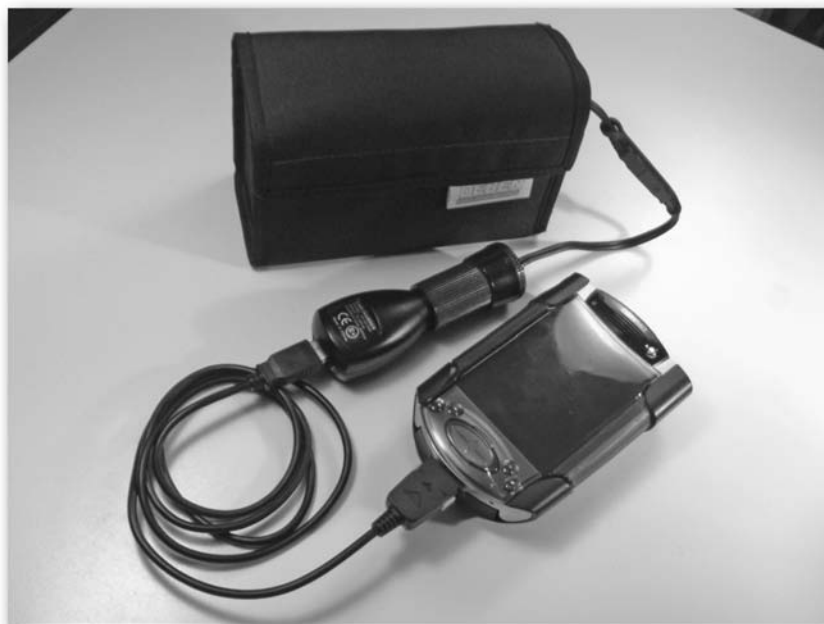
FIGURE 11-23: Portable lead-acid battery wiley.HACKING.GPS.MAR.2005.EBOOK-LING
