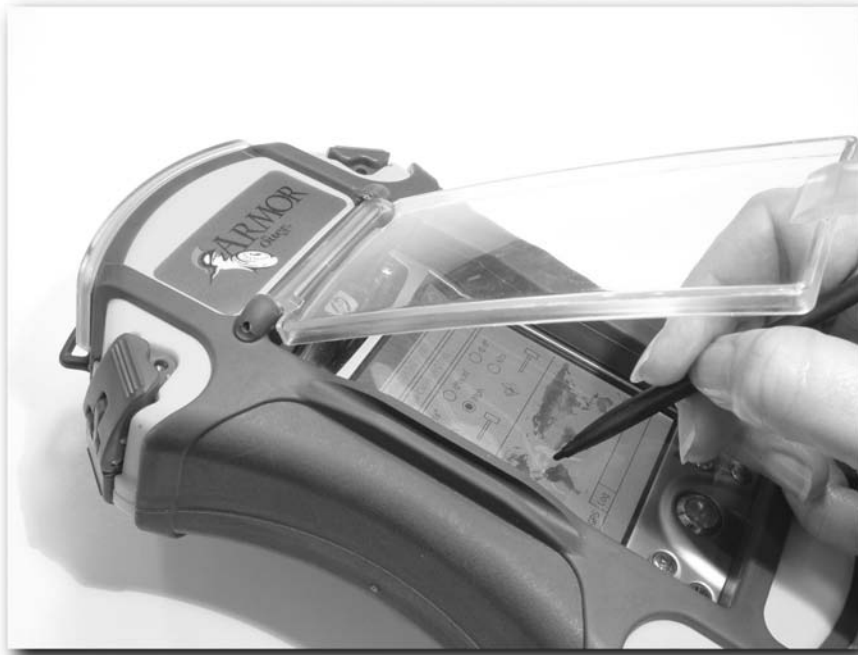
FIGURE 5-28: The well-armored Otter 3600 has a flip-down polycarbonate covering to shield the plastic film on the front.
