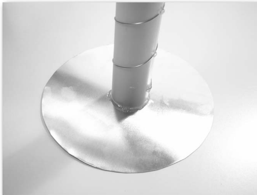
FIGURE 4-18: Epoxy resin is great for attaching the helix coil base to the ground plane.
