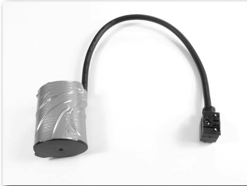
FIGURE 3-19: Completed film pot battery holder
