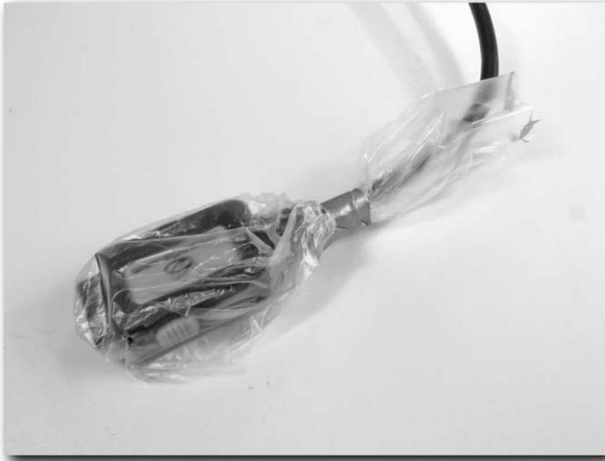
FIGURE 11-18: Connector protected by a small plastic bag
