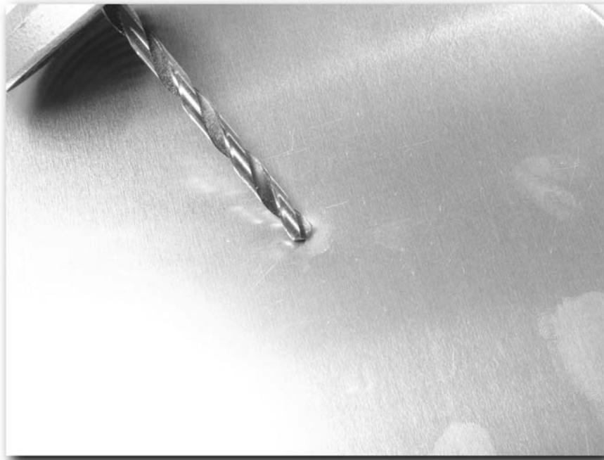
FIGURE 4-15: Cutting the hole in the metal sheet that will become the ground plane
