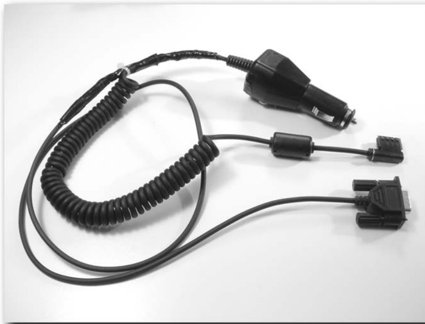
FIGURE 2-4: A combo cable combines data and power functions.
