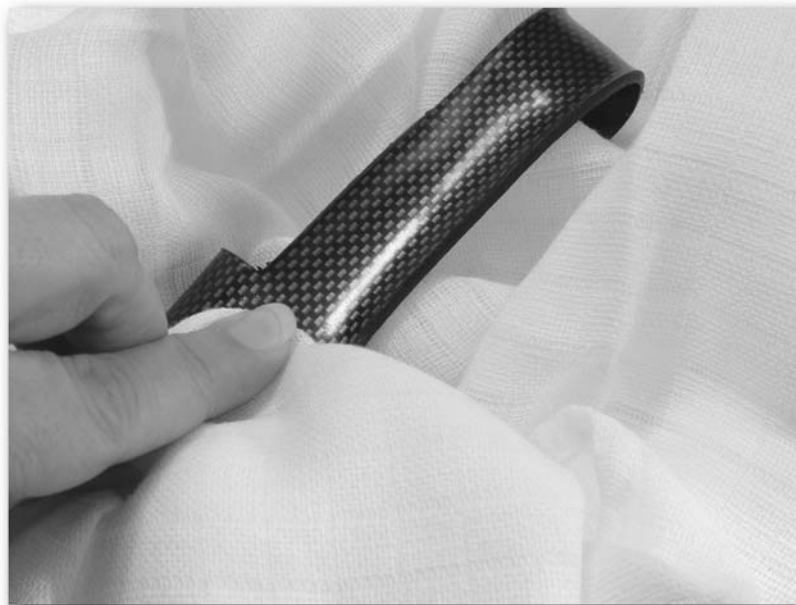
FIGURE 5-41: Damp cloths enable you to selectively cool down areas of the plastic quickly, minimizing the time you have to hold it in place.
