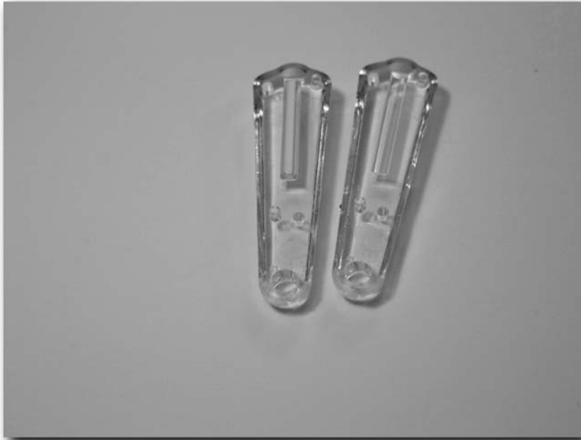
FIGURE 11-31: Splitting the outer case of the Glowring
