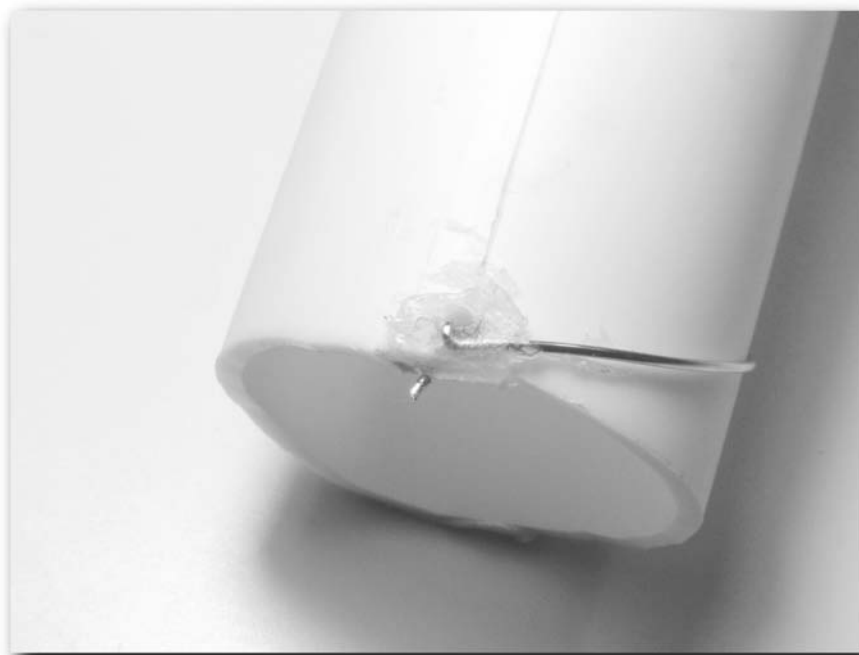
FIGURE 4-20: Holding the wire in place at the top
