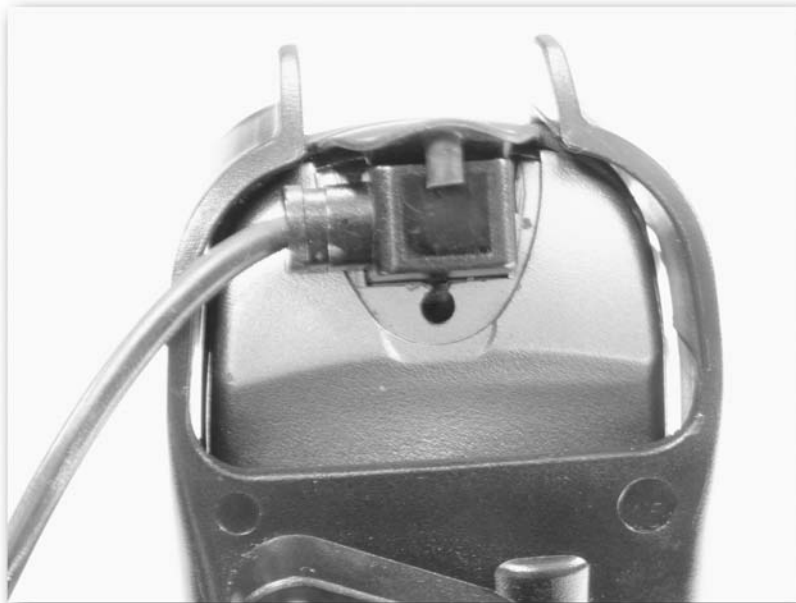
FIGURE 5-32: This cradle enables you to attach a cable connector to the GPS, an option not available with all mounts.
