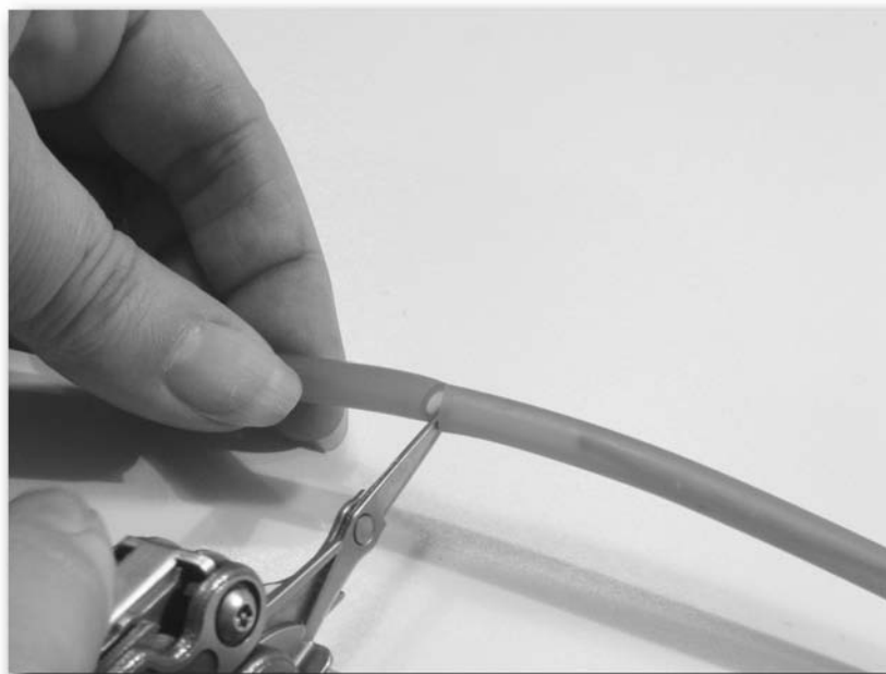
FIGURE 5-14: Make sure that the tubing extends over any sharp edges.
