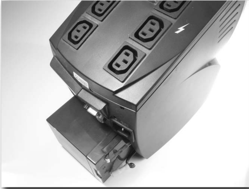
FIGURE 3-6: A lead-acid battery from a UPS device
