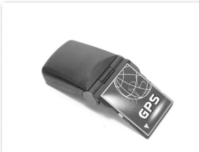
FIGURE 7-2: The Haicom HI-401 foldable GPS receiver and a Haicom Bluetooth connecting slipper wiley.HACKING.GPS.Mar.2005.EBOOK-LING
