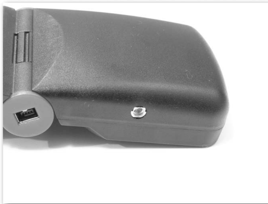
FIGURE 4-9: MMCX connector on a Haicom Compact Flash GPS
