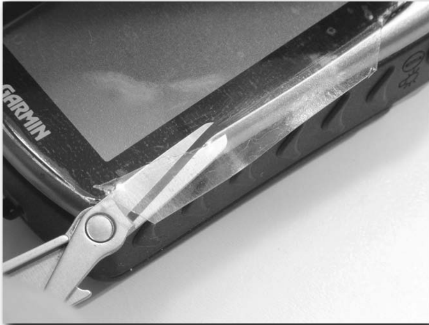
FIGURE 5-7: Carefully cut around the edges of the screen protector.
