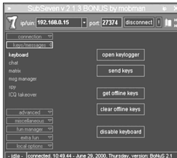
Figure 15.8. Keyboard window that enables the attacker to control the victim's key strokes.
