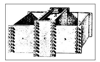
**Figure 1-6.** French Caisson. This caisson could be floated over the work site and lowered to the bottom by flooding the side tanks.
