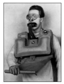
**Figure 1-10.** Original Davis Submerged Escape Apparatus.
