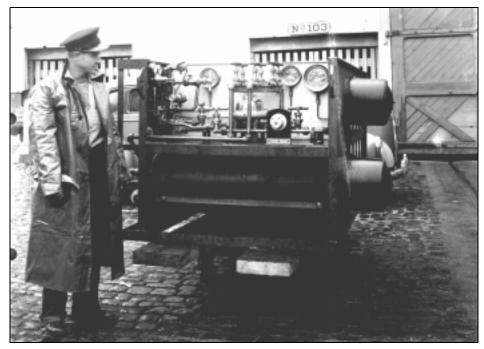
Figure 1-14. Helium-Oxygen Diving Manifold.
