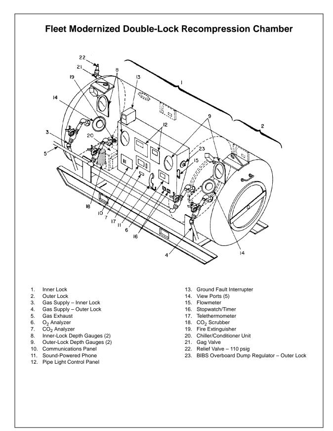
Figure 22-4. Fleet Modernized Double-Lock Recompression Chamber.
