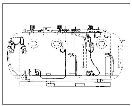
Figure 22-9. Fly Away Recompression Chamber.
