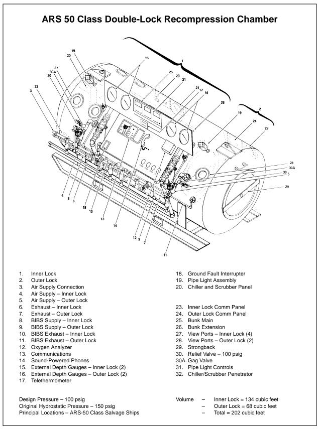
Figure 22-3. ARS 50 Class Double Lock Recompression Chamber.
