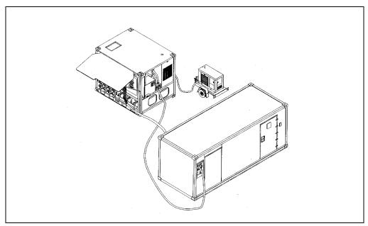
Figure 22-8. Fly Away Recompression Chamber (FARCC).
