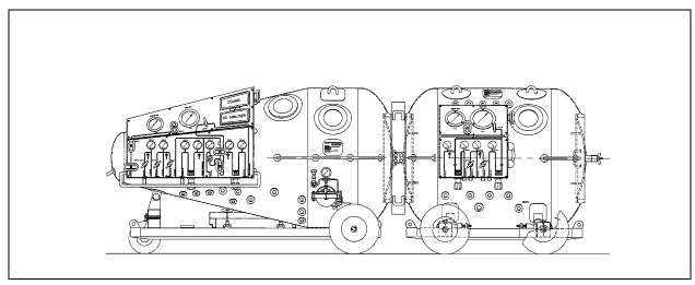
Figure 22-5. Transportable Recompression Chamber System (TRCS).
