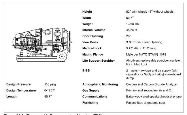
**Figure 22-6.** Transportable Recompression Chamber (TRC).
