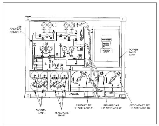
Figure 22-10. Fly Away Recompression Chamber Life Support Skid.
