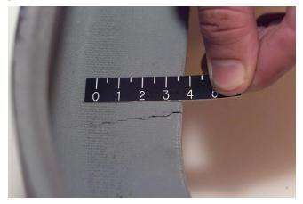
For the panel 6L test, a 20,000-cm3 BX 250 foam projectile impacted the panel at a velocity of 234 m/sec. A lower corner of the foam block first impacted the panel near the slip-side rib. The resulting crack, which measured approximately 14 cm, traversed the entire rib and lock and 1.9 cm onto the lower panel face. In addition, the panel 6L T-seal exhibited a crack 6.4 cm along its web.
