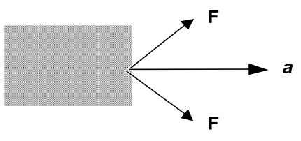
Figure 1 The acceleration produced by two forces is in the direction of the vector sum of the forces.
