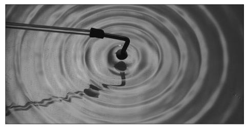
Cylindrical wave pattern produced in a ripple tank. When not modified by the no-slip condition at solid surfaces, waves are nearly inviscid and well represented by the potential theory of this chapter. (*Courtesy of Dr. E. R. Degginger/Color-Pic Inc.*)
