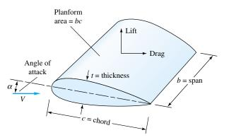
**Fig. 7.22** Definition sketch for a lifting vane.
