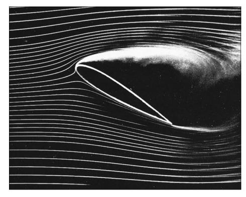
Fig. 7.24 At high angle of attack, smoke-flow visualization shows stalled flow on the upper surface of a lifting vane. [From Ref. 19, Illustrated Experiments in Fluid Mechanics (The NCFMF Book of Film Notes), National Committee for Fluid Mechanics Films, Education Development Center, Inc., copyright 1972.]
