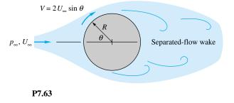
the separated flow on the rear, the pressure is assumed equal to its value at  $\theta = 90^{\circ}$ . Compute the theoretical drag coefficient and compare with Table 7.2.
