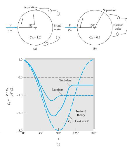
**Fig. 7.13** Flow past a circular cylinder: (*a*) laminar separation; (*b*) turbulent separation; (*c*) theoretical and actual surface-pressure distributions.
