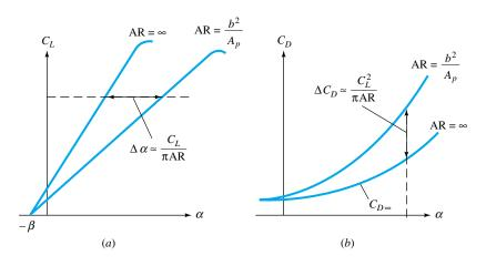
**Fig. 7.27** Effect of finite aspect ratio on lift and drag of an airfoil: (*a*) effective angle increase; (*b*) induced drag increase.
