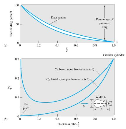
**Fig. 7.12** Drag of a streamlined two-dimensional cylinder at  $\text{Re}_c = 10^6$ : (*a*) effect of thickness ratio on percentage of friction drag; (*b*) total drag versus thickness when based upon two different areas.
