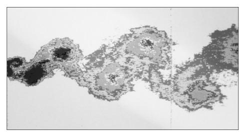
The turbulent wake behind a bluff body immersed in a stream flow is a subject of the present chapter. This is a digitized video image showing the distribution of tracer-dye concentration in the wake of the body. Compare with Fig. 5.2a of the text, which is a laminar wake. (*Courtesy of R. Balachandar, by permission of the American Society of Mechanical Engineers.*)
