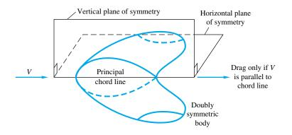
The Reynolds number is based upon the free-stream velocity V and a characteristic length L of the body, usually the chord or body length parallel to the stream
