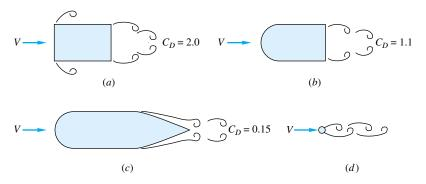
Fig. 7.15 The importance of streamlining in reducing drag of a body ( $C_D$  based on frontal area): (*a*) rectangular cylinder; (*b*) rounded nose; (*c*) rounded nose and streamlined sharp trailing edge; (*d*) circular cylinder with the same drag as case (*c*).
