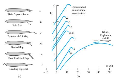
Fig. 7.28 Performance of airfoils with and without high-lift devices: A = NACA 0009; B = NACA 63-009; C = Kline-Fogleman airfoil (from Ref. 17); D to I shown in (a): (a) types of high-lift devices; (b) lift coefficients for various devices.
