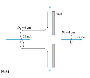
passes through the hole, and part is deflected. Determine the horizontal force required to hold the plate.
