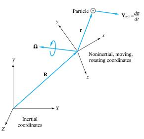
**Fig. 3.12** Geometry of fixed versus accelerating coordinates.
