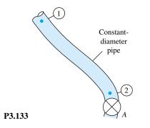
What is the friction head loss between 1 and 2, in m, for the flowing condition?
