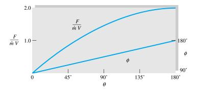
These can be plotted versus  $\theta$  as shown in Fig. E3.9. Two special cases are of interest. First, the maximum force occurs at  $\theta = 180^\circ$ , that is, when the jet is turned around and thrown back in the opposite direction with its momentum completely reversed. This force is 2mV and acts to the *left*; that is,  $\phi = 180^{\circ}$ . Second, at very small turning angles ( $\theta < 10^{\circ}$ ) we obtain approximately
