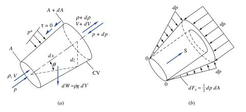
**Fig. 3.15** The Bernoulli equation for frictionless flow along a streamline: (*a*) forces and fluxes; (*b*) net pressure force after uniform subtraction of p. This relation does not require an assumption of frictionless flow.
