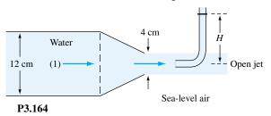
If the pressure at the centerline at section 1 is 110 kPa, and losses are neglected, estimate (a) the mass flow in kg/s and (b) the height H of the fluid in the stagnation tube.
