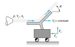
the power P delivered to the cart. Also find the cart velocity for which (c) the force  $F_x$  is a maximum and (d) the power P is a maximum.
