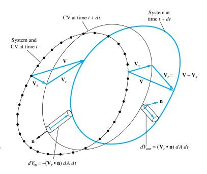
Fig. 3.5 Relative-velocity effects between a system and a control volume when both move and deform. The system boundaries move at velocity V, and the control surface moves at velocity  $V_s$ .
