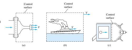
**Fig. 3.2** Fixed, moving, and deformable control volumes: (*a*) fixed control volume for nozzle-stress analysis; (*b*) control volume moving at ship speed for drag-force analysis; (*c*) control volume deforming within cylinder for transient pressure-variation analysis.
