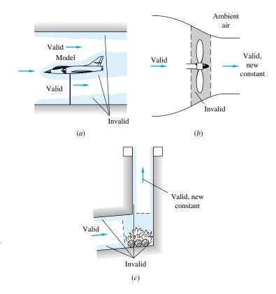
**Fig. 3.16** Illustration of regions of validity and invalidity of the Bernoulli equation: (*a*) tunnel model, (*b*) propeller, (*c*) chimney.
