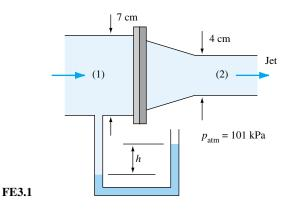
friction is neglected, what is the axial flange force required to keep the nozzle attached to pipe 1?
