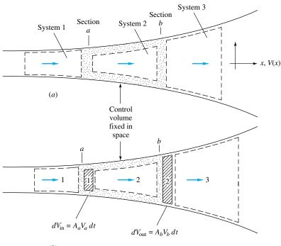
**Fig. 3.3** Example of inflow and outflow as three systems pass through a control volume: (*a*) System 2 fills the control volume at time t; (*b*) at time t + dt system 2 begins to leave and system 1 enters.
