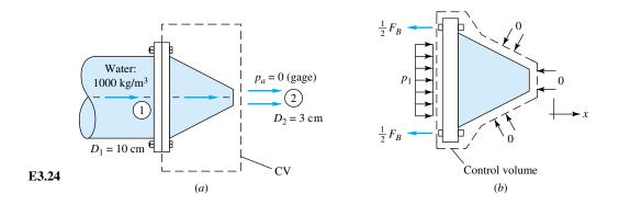
The velocities are found from the known flow rate  $Q = 1.5 \text{ m}^3/\text{min}$  or 0.025 m<sup>3</sup>/s:
