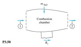
tion 2 at atmospheric pressure and higher temperature, where  $V_2 = 900$  m/s and  $A_2 = 0.4$  m<sup>2</sup>. Compute the horizontal test stand reaction  $R_x$  needed to hold this engine fixed.
