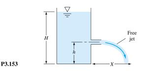
leaving horizontally will strike the floor, as a function of h and H. For what ratio h/H will X be maximum? Sketch the three trajectories for h/H = 0.4, 0.5, and 0.6.
