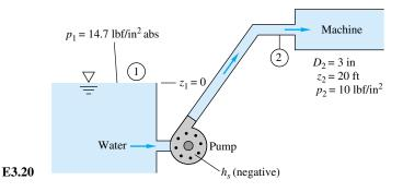
where  $K \approx 7.5$  is a dimensionless loss coefficient (see Sec. 6.7). Take  $\alpha \approx 1.07$ . Find the horsepower required for the pump if it is 80 percent efficient.
