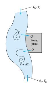
**P3.128** For the conditions of Prob. 3.127, if the power plant is to heat the nearby river water by no more than 12°C, what should be the minimum flow rate Q, in m<sup>3</sup>/s, through the plant heat exchanger? How will the value of Q affect the downstream conditions ( $Q_0$ ,  $T_0$ )?
