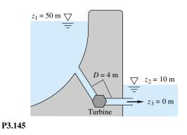
pipe. For what river flow rate in  $m^3/s$  will the power extracted be 25 MW? Which of the *two* possible solutions has a better "conversion efficiency"?
