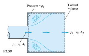
corners and the flow gradually expands to  $A_2$  downstream. Using the suggested control volume for incompressible steady flow and assuming that  $p \approx p_1$  on the corner annular ring as shown, show that the downstream pressure is given by
