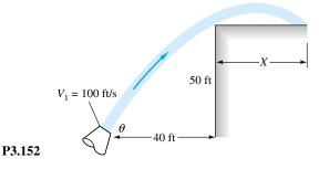
**P3.153** For the container of Fig. P3.153 use Bernoulli's equation to derive a formula for the distance X where the free jet
