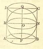
two bases, each of which is equal to a great circle, we have the entire surface of the cylinder equal to six great circles: hence, the surface of the sphere is to the entire surface of lie circumscribed cylinder, as 4 is to 6, or as 2 is to 3; which was to be proved.
