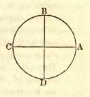
the secondary diameter; the point A, from which arcs are usually reckoned, is called the origin of arcs, and the point B, 90° distant, is called the secondary origin. Arcs estimated from A, around towards B, that is, in a direction contrary to that of the motion of the hands of a watch, are considered positive; consequently, those reckoned in a contrary direction must be regarded as negative.
