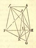
The remaining pyramid may be regarded as having the triangle FfH for its base, and the point g for its vertex. From g, draw gK parallel to fF, and draw also KH and Kf. Then will the pyramids K-FfH and g-FfH, be equal; for they have a common base, and their altitudes are equal, because their vertices K and g are in a line parallel to the base (B. VI., P. XII., C. 2).
