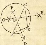
Scholium. The same construction enables us to pass a circumference through any three points not in a straight line. If the points are vertices of a triangle, the circle will be circumscribed about it.
