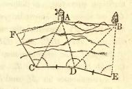
equal to 200 yards; from the former of these points, A could be seen, and from the latter, B; and at each of the points C and D, a staff was set up. From C, a distance CF was measured, not in the direction DC, equal to 200 yards, and from D, a distance DE, equal to 200 yards, and the following angles taken:
