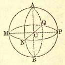
of division with the points A and B, by a quadrant: there will be formed 96 equal isosceles spherical triangles (P. VII., S. 2) on the surface of the sphere, of which the lune will contain 10: hence, in this case, the area of the lune is to the surface of the sphere, as 10 is to 96, or as 5 is to 48; that is, as the arc MN is to the circumference MNPQ, or as the angle of the lune is to four right angles.
