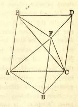
altitude, because their bases are in the same plane AD, and their vertices at the same point F; hence, they are equal in volume (P. XV.). The pyramids ABC-F and DEF-C, have their bases ABC and DEF, equal because they are the bases of the given prism, and their altitudes are equal because each is equal to the altitude of the prism; they are, therefore, equal in volume: hence, the three pyramids into which the prism is divided, are all equal in volume; which was to be proved.
