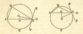
For, the angle ABF, equal to EBD, is measured by half of the arc AKB (P. XXI.); and the inscribed angle AMB is measured by half of the same arc: hence, the angle AMB is equal to the angle EBD, and consequently, to the given angle.
