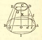
the convex surface of the frustum of the pyramid coincides with that of the cone, the perimeters of its bases coincide with the circumferences of the bases of the frustum of the cone, and its slant height is equal to that of the cone: hence, the convex surface of the frustum of a cone is equal to half the sum of the circumferences of its bases multiplied by the slant height; which was to be proved.
