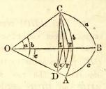
CD and CE, these lines will be respectively perpendicular to OA and OB (B. VI., P. VI.), and the angles CDP and CEP will be equal to the angles A and B respectively. Draw DL and PQ, the one perpendicular, and the other parallel to OB. We then have,
