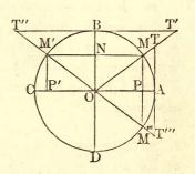
AOM and AOM''', are also equal. The right-angled triangles AOT and AOT''', have a common base AO, and the angles at the base equal; consequently, the remaining parts are respectively equal: hence, AT is equal to AT'''. But AT is the targent of AM, and AT''' is the targent of AM': hence, the tangent of an arc is equal to the tangent of its supplement.
