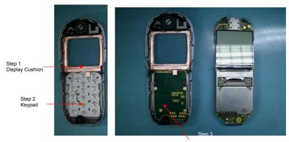
Photo 2.20 Keypad and Display cushion assembly
