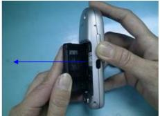
Photo 2.4. Battery compartment
