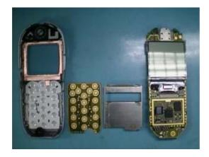
Photo 2.10 Keypad PCB and Shield removing
