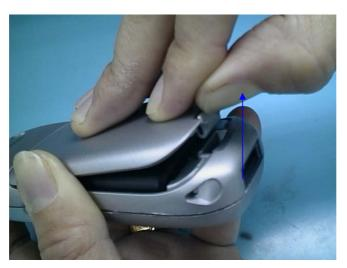
Photo 2.3 Battery cover removing
