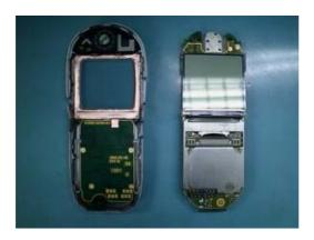
Photo 2.9 RF board removing
