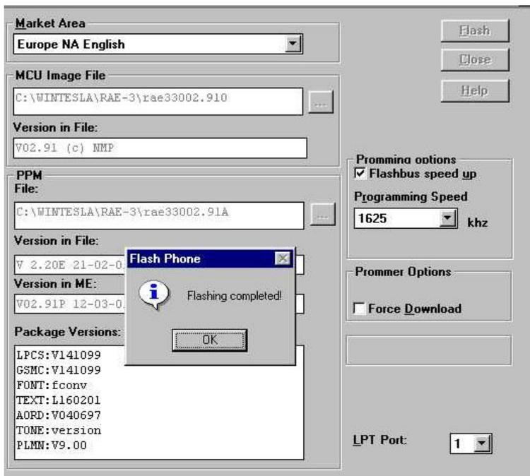
Figure 11. Flash programming completed
