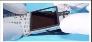
8. The Display Shield is hooked at its bottom side.
