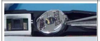
5. The Earpiece is stuck with double-sided adhesive tape. Use new tape when mounting the Speaker.
