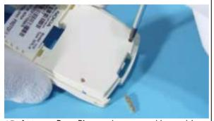
15. Antenna Pogo Pins can be removed by pushing them with torx driver through the C-Cover.
