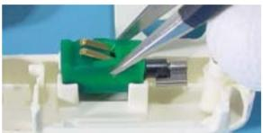
12. Grip the Vibra Motor at the rubber and pull it off from its quidance.
