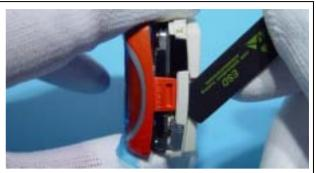
2. Unlock the top guidance to remove the A-Cover.
