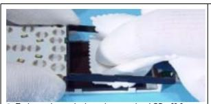
9. Take a clean cloth and press the *LCD* off from the *LCD Frame*.
