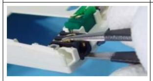
11. To remove the *DC Jack*, insert tweezers between the spring contacts and under the jack. You need to use some force to pull the jack upwards.
