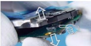
4. Take the modules from the C-Cover and unplug the display connector by pulling the modules apart carefully.
