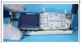
3.Unscrew the six T6 screws, using the shown order. For assembly, the reverse order and a torque of 17Ncm have to be used.
