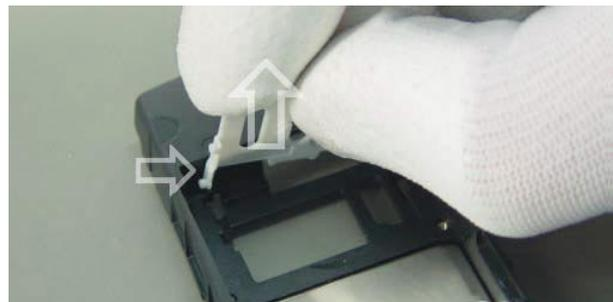
The second step is to push one hinge to the middle to lift up the Card Cover.
