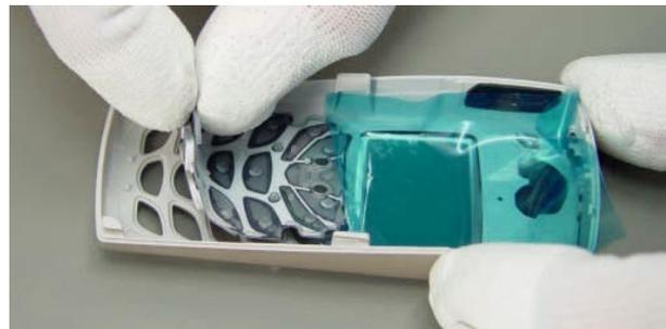
Grab the Keymat and remove it. It is always good to protect the window also from the inner side.
