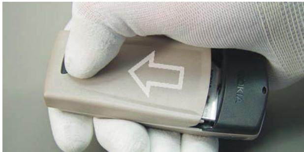
Push the unlock-button and move the battery cover in direction to the System Connector.
