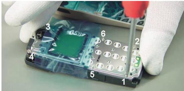
**Remove the six screws with screwdriver Torx T6 in the shown order. When assembling the reverse order has to be taken with a torque of 17Ncm.**
