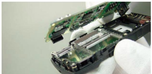
Lift up the CMT module LA5 carefully. Sometimest it happens that the battery connector gets stuck at the SIM CardCover. Take care not to bend the spring contacts of the battery connector.
