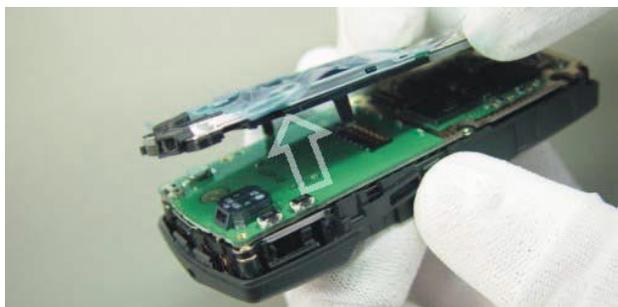
Now the UI module can be removed. Please take care not to damage the board to board connector afterwards which is located on the CMT module.
