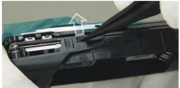
Before removing the UI module LU9 this clip has to be released with a screwdriver or tweezers.
