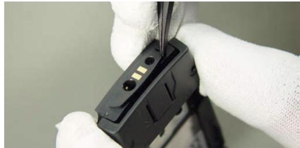
Turn around the B-Cover. If the System Connector is jammed, press with tweezers between cover and connector.
