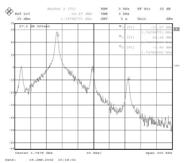
The purpose of this tuning is to tune the carrier signal and the +67kHz signal to a minimum level (Marker 2 and 3).
