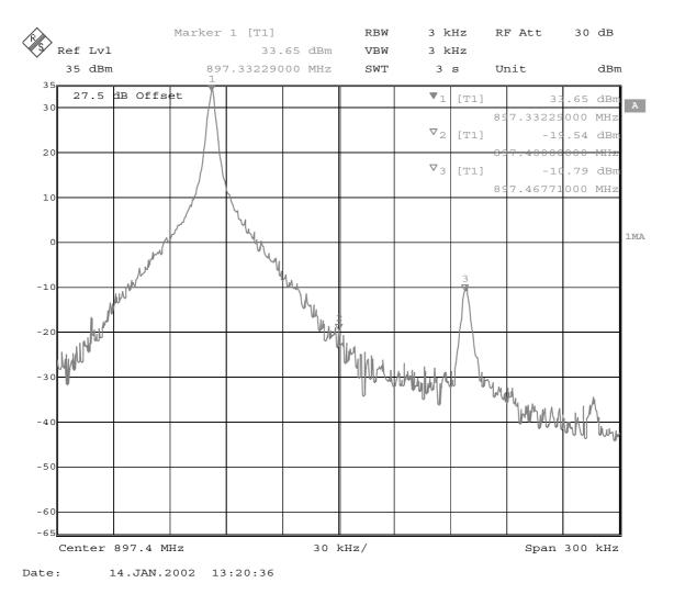
Use the variables 'Amplitude difference' and 'Phase difference' to adjust the +67kHz signal to a minimum level (Marker 3). After tuning to the minimum the level difference between the peak levels at marker 1 and 3 must exceed 40dB. Tuning is possible by using arrow keys on the keyboard. Pushing the sliders by using the mouse is less sensitive but even possible.
