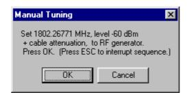
Connect an external signal generator to the RF connector of the phone and set the generator as told in the window.
