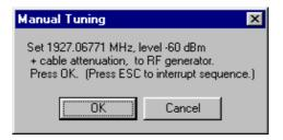
Connect an external signal generator to the RF connector of the phone and set the generator as told in the window.
