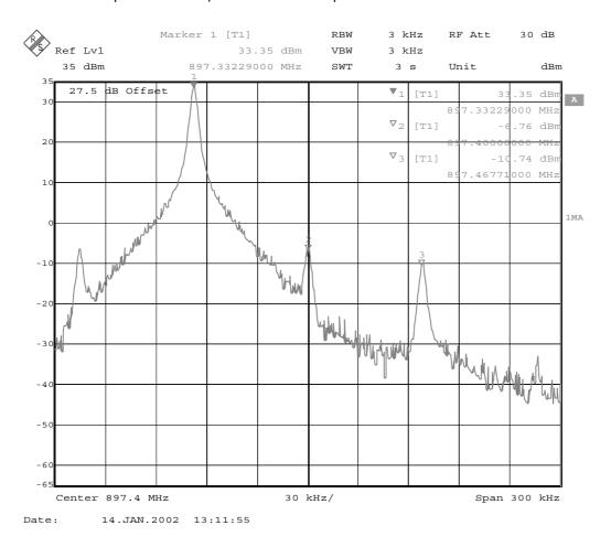
The purpose of this tuning is to tune the carrier signal and the +67kHz signal to a minimum level (Marker 2 and 3).
