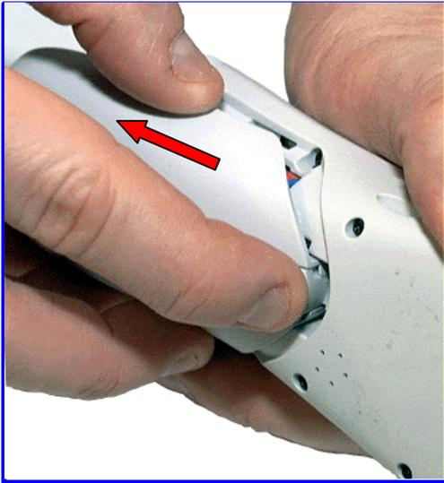
1. Remove battery door by pressing down on latch and pulling back
