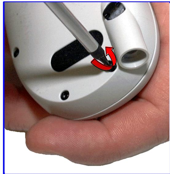
4. Unscrew 6 retaining screws using T6 Torx driver – find screw locations on page 4
