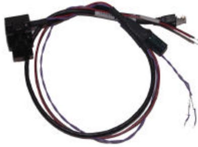
**Fig 6.3** Flash Cable (with Power leads)
