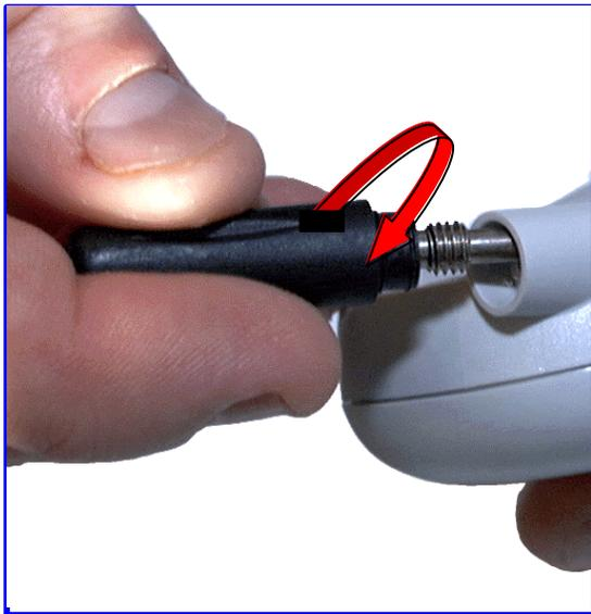
3. Remove antenna by rotating anti-clockwise
