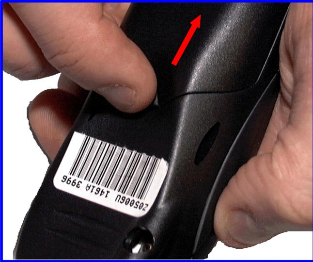
1. Remove battery door by pressing down on latch and pulling back
