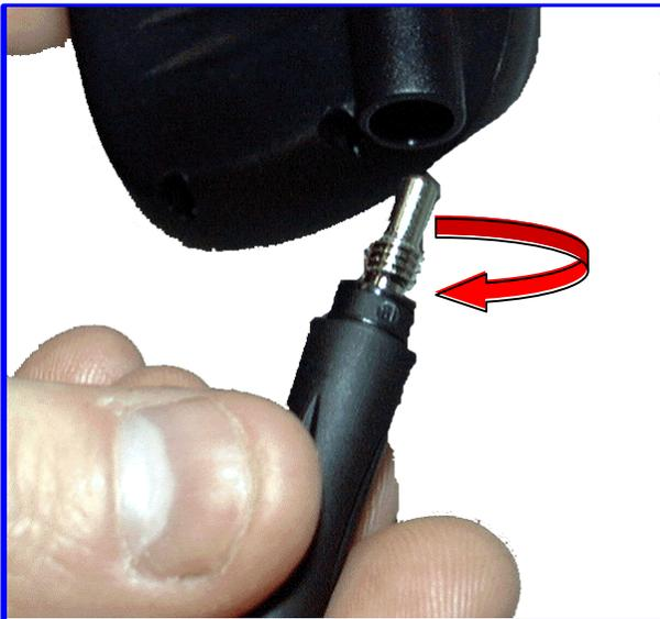
3. Remove antenna by rotating anti-clockwise
