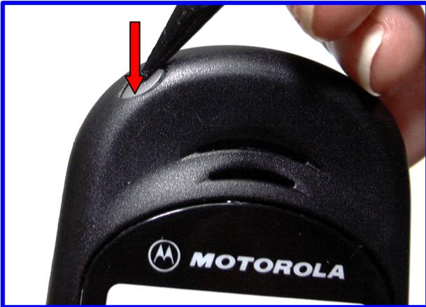
15. Carefully press down on Service Indicator, if it gets damaged / scratched during this process, replace.
