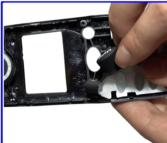
13. Remove keypad from front housing
