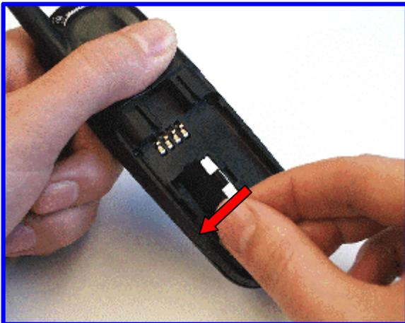
3. Press down and push SIM cover to the left, then remove SIM card.
