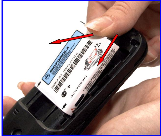
2. Remove battery by pushing and lifting at the same time.
