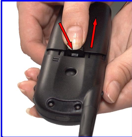
1. Remove battery door by pressing down on clip and sliding back.
