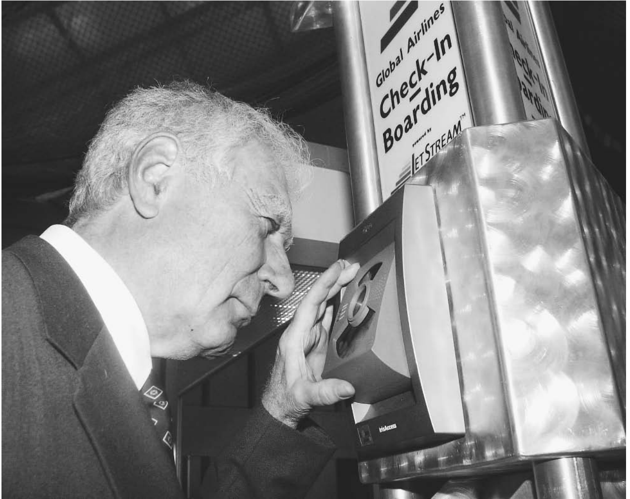
An executive demonstrates a retinal scanner used for identification at the International Air Transport Association security symposium in Atlanta in 2001. AP/WIDE WORLD PHOTOS.
