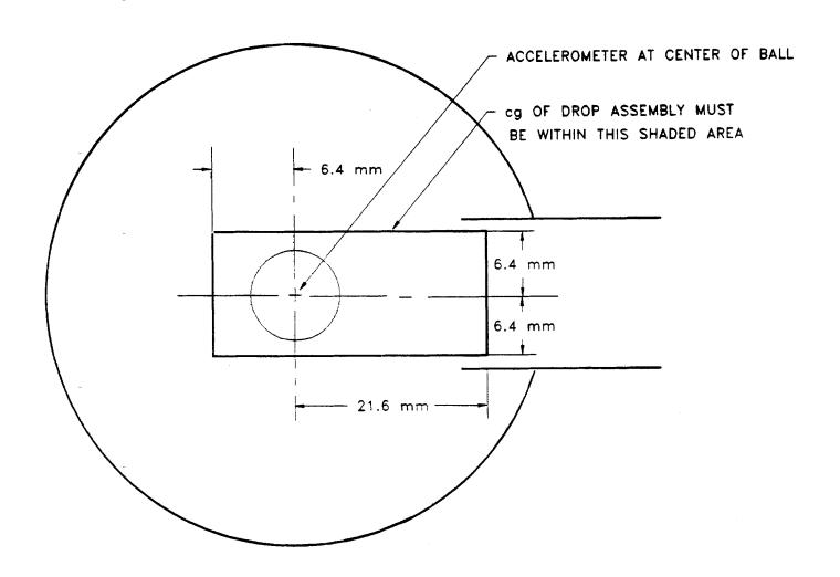
Figure 10. Center of Gravity for Drop Assembly
