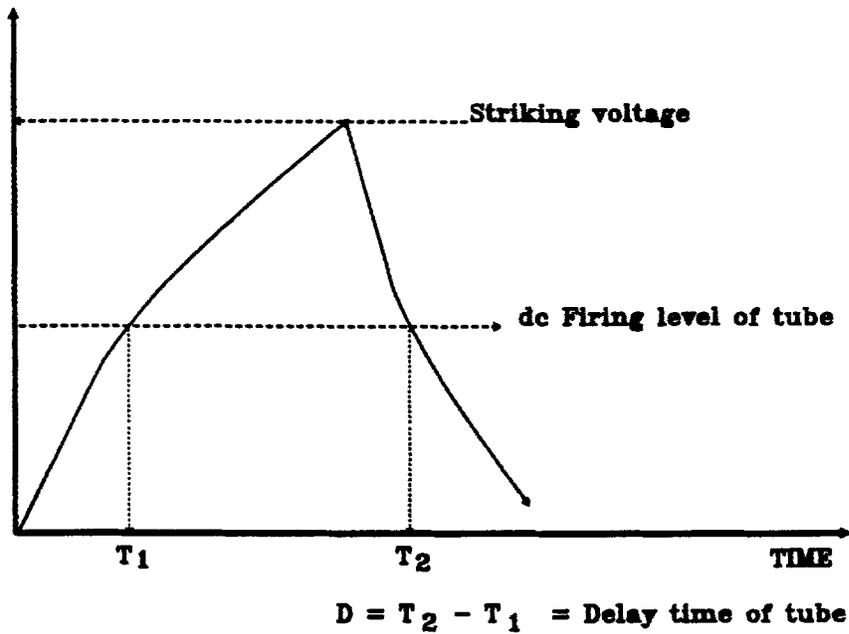
**Note:** The delay time is that period of time when the potential across an arrester exceeds its dc firing level.
