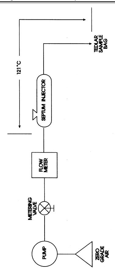
FIGURE M90-1 APPARATUS FOR PREPARATION OF FID METHANOL RESPONSE CALIBRATION MIX
