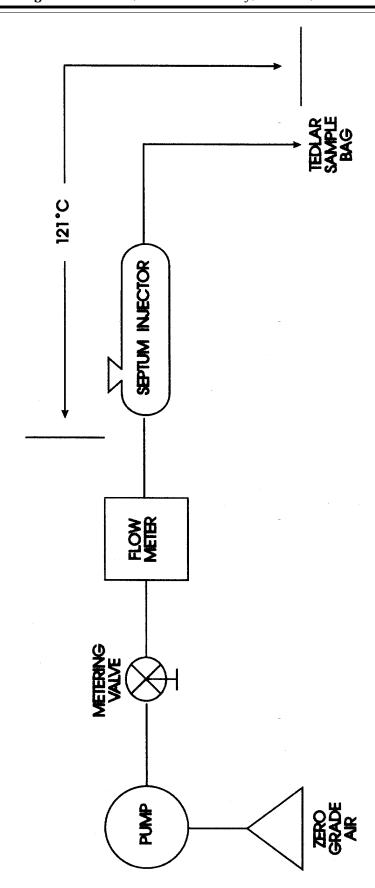
FIGURE 890-11 APPARATUS FOR PREPARATION OF FID METHANOL RESPONSE CALIBRATION MIX
