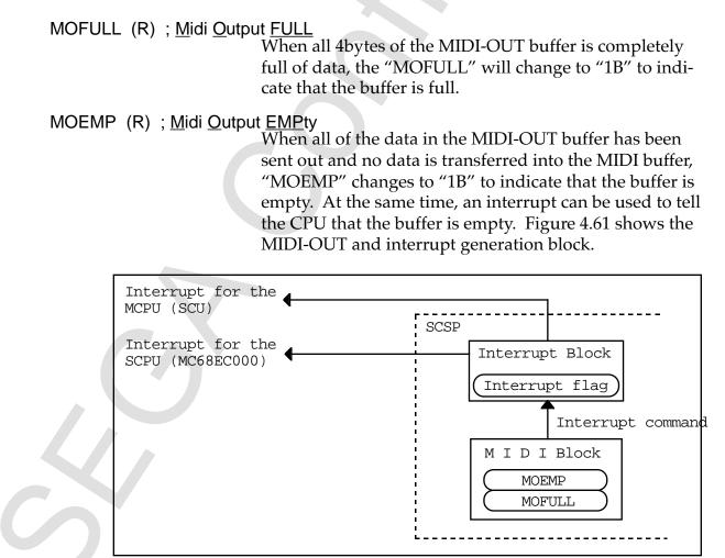
Figure 4.61 MIDI OUT Block and the Interrupt Generation Block
