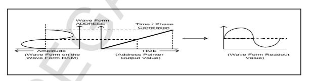
Figure 4.20 Creating Wave Form Addresses and Reading Wave Form Data
