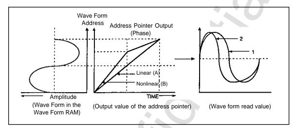
Figure 4.24 Frequency Address Pointer Output Value During FM Voice Mixing Execution (2)
