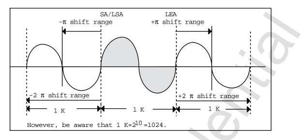
Figure 4.40 Address Shift during FM Voice Synthesis
