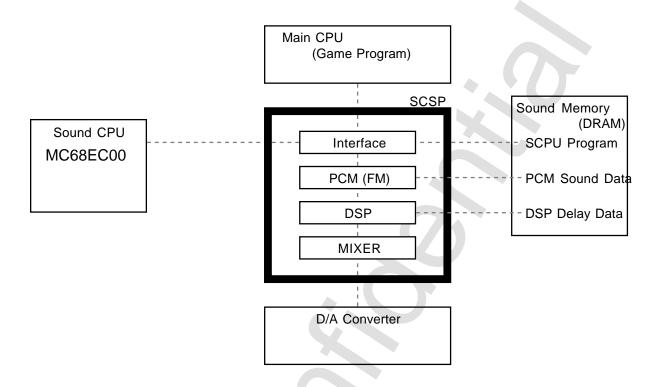
Figure 1.2 Sound System Configuration
