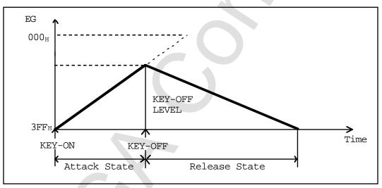
Figure 4.12 KEY\_OFF During Attack State Transition
