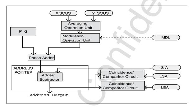
Figure 4.19 Wave Form Address Generator
