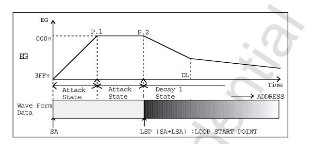
Figure 4.15 Transition (1) from the Attack State to Decay 1
