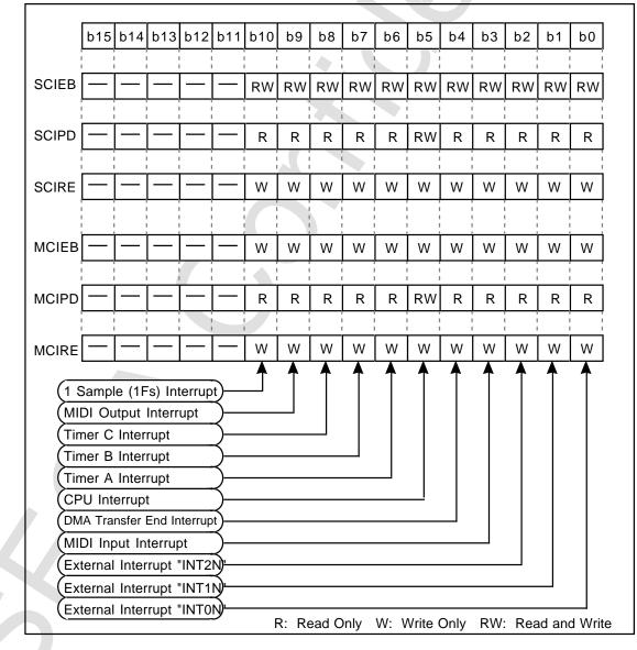
Figure 4.63 Interrupt Register Bit Accommodation
