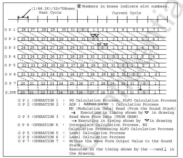
Figure 4.30 Slot Calculation and Sound Stack State
