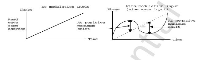
Figure 4.39 Maximum Shift of the Wave Form Read Address
