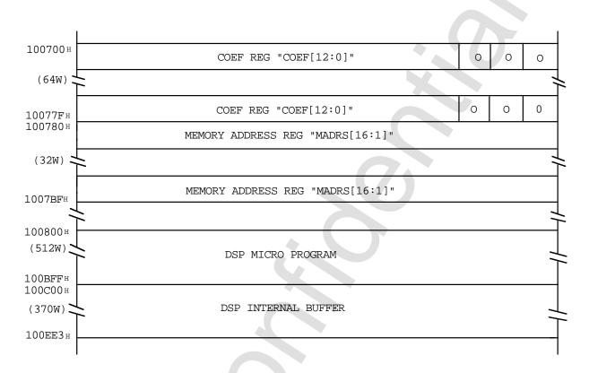
Figure 4.5 DSP Control Register
