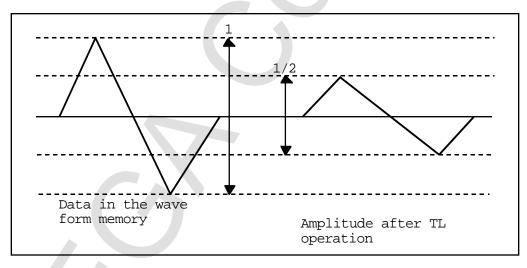
Figure 4.50 Wave Data when TL bit 4 = 1
