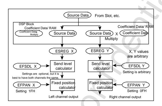
Figure 4.55 DSP Panning Calculation
