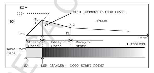
Figure 4.16 Transition (2) from the Attack State to Decay 1
