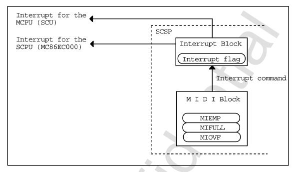
Figure 4.60 MIDI IN Block and the Interrupt Generation Block
