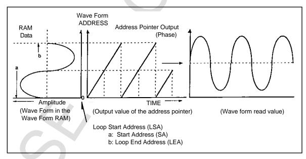
Figure 4.23 Address Pointer Output Value During FM Voice Mixing Execution(1)
