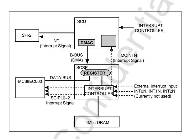
Figure 4.62 Sound Interrupt Signal Connections Diagram
