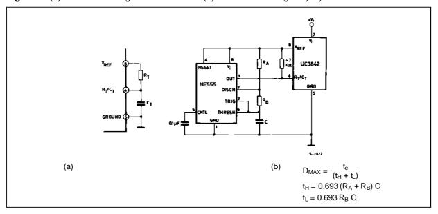
Figure 8: Synchronization to an External Clock.
