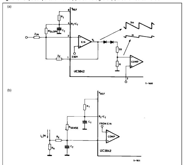
Figure 20: Slope Compensation Added (a) to Control Signal or (b) to Current Sense Waveform.
