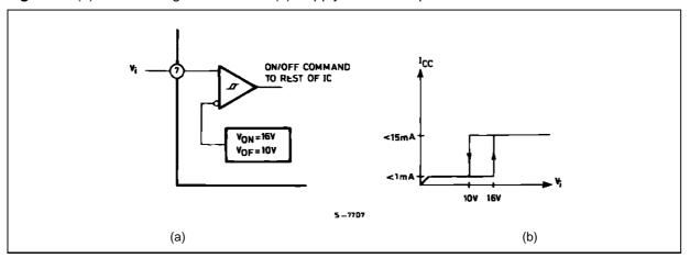
Figure 6: Providing Power to the UC3842.
