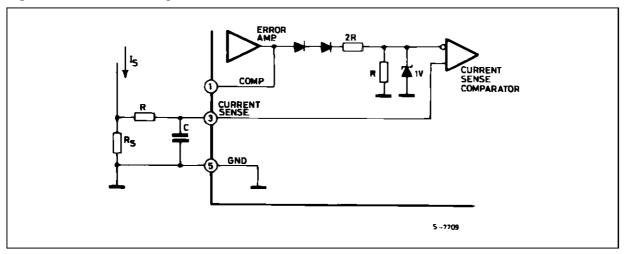
Figure 13: Transformer-coupled Current Sensing.
