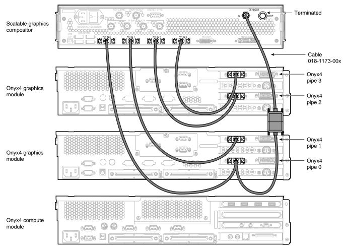
Figure 3-4 Connecting the DVI and Genlock In Connectors
