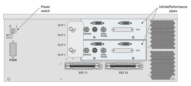
Figure 4-7 V-brick with Two InfinitePerformance Pipes
