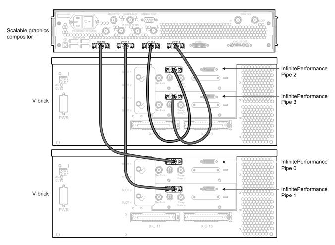
Figure 4-9 Connecting the DVI Connectors
