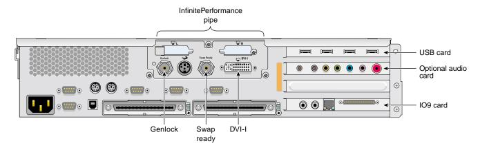
Figure 4-1 SGI Onyx 350 Compute/Graphics Module with One InfinitePerformance Pipe
