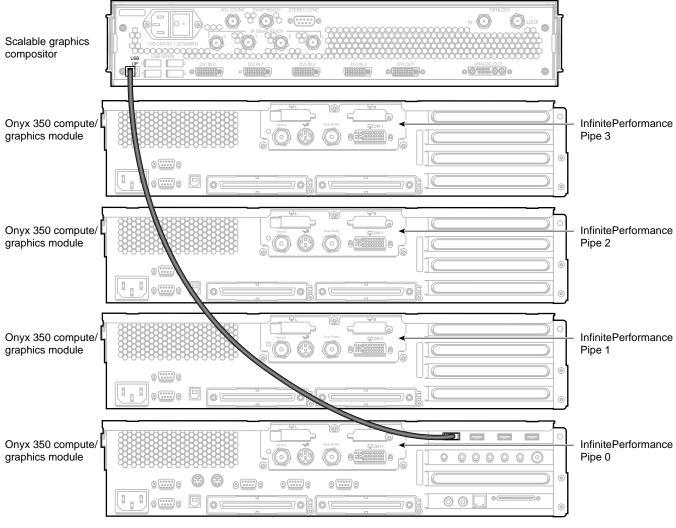
Figure 4-3 Connecting the USB Connectors
