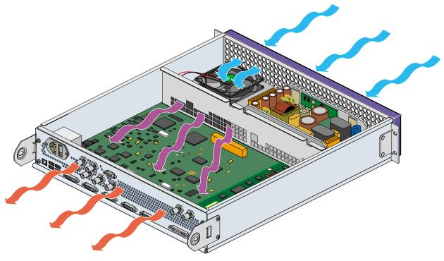
Figure 1-5 Chassis Airflow Diagram
