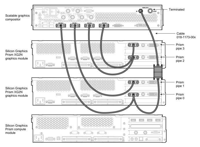
Figure 2-4 Connecting the DVI and Genlock In Connectors
