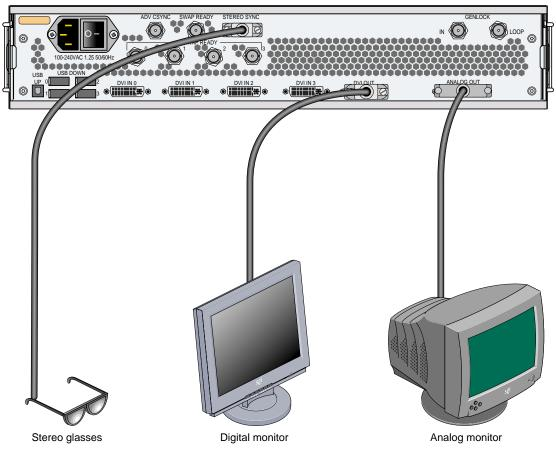
Figure 1-4 Example Connections to Digital and Analog Display Devices
