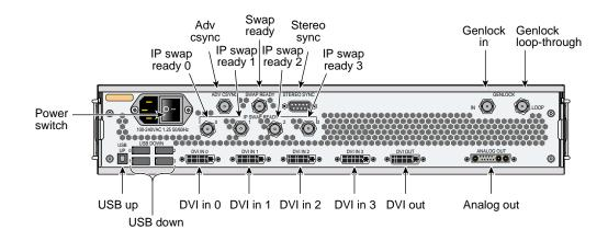
Figure 1-3 Rear Panel of the Scalable Graphics Compositor
