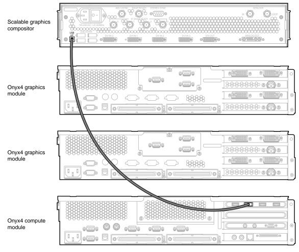
3. Using a USB cable, connect the **USB UP** port on the compositor to a USB connector port on the USB PCI option card installed in the Onyx4 compute module (as shown in Figure 3-3):
