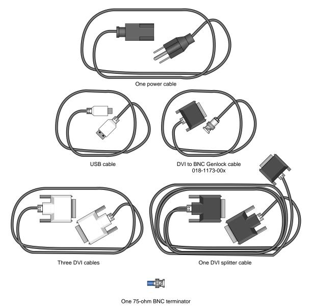
Figure 2-2 Cables and Other Cabling Items Needed for Installation
