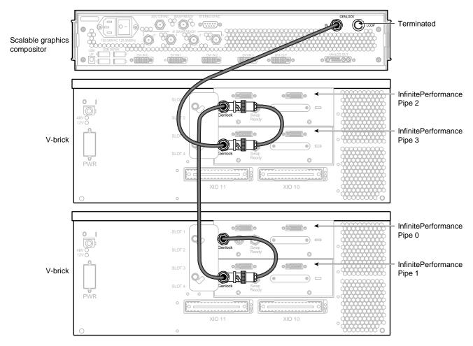
Figure 4-11 Connecting the Genlock Connectors
