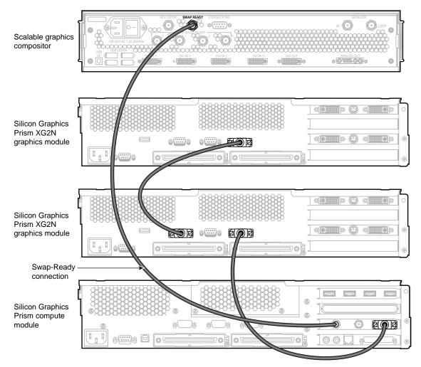
7. Connect an additional image sync cable from the **Repeat** connector to the image sync **IS1** connector on the next XG2N graphics module.
