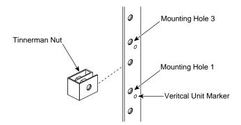
Figure 1-1 Installing a Timmerman Nut to a Mounting Hole
