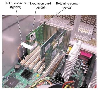
Figure 9-8 Installed Expansion Cards
