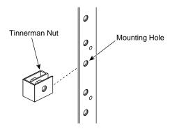
Figure 1-6 Installing a Timmerman Nut to a Mounting Hole
