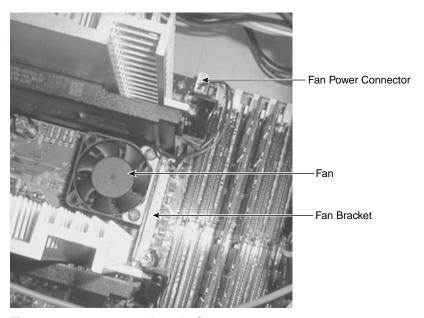
Figure 9-16 Processor Area Cooling Fan
