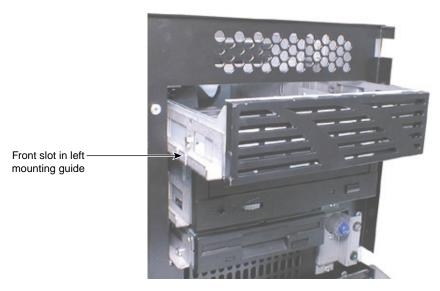
Figure 9-5 Inserting Device Tray
