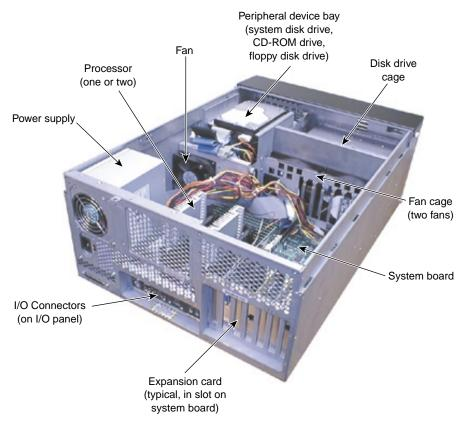
Figure 7-2 Internal System Components
