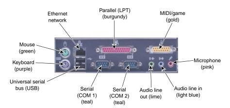
Figure 1-10 Input/Output (I/O) Panel
