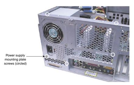
**Figure 9-11** Power Supply Mounting Screws
