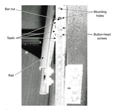
Figure 1-5 Rail Secured to FrontMounting Rail on Equipment Rack
