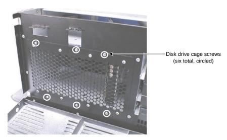
Figure 9-6 Disk Drive Cage Installed
