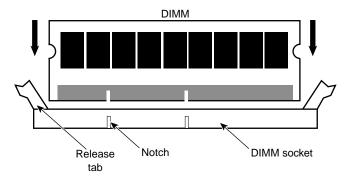
Figure 9-9 Dual Inline Memory Module (DIMM)
