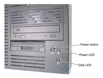
Figure 4-1 System Power Button and LEDs
