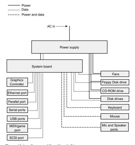
Figure 10-1 Power and Data Signals Diagram
