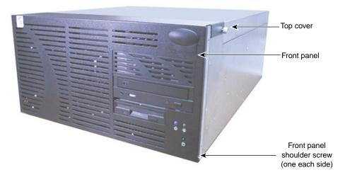
Figure 9-1 Base Unit Chassis Components
