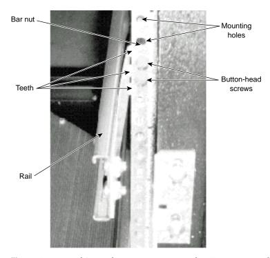
Figure 1-7 Rail Secured to Rear Mounting Rail on Equipment Rack
