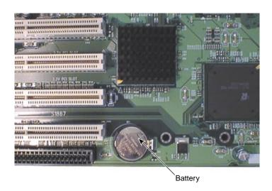
Figure 9-18 CMOS/Clock Lithium Battery
