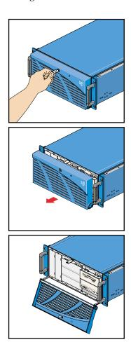
Figure 3 Opening a Node Bezel
