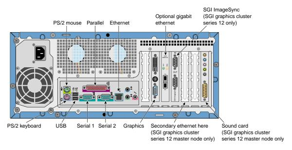
Figure 2 Rear Panel I/O Ports and Features
