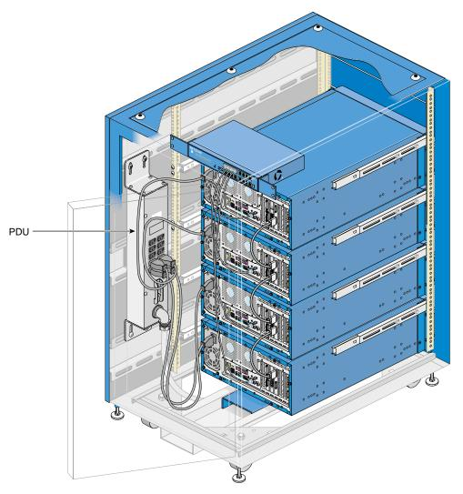
Figure 1 Rack PDU and Node Cables
