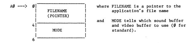
The sound and video buffers are constantly scanned by the Macintosh hardware to determine what sounds to emit from its speakers and what to display on its screen. (The video buffer is the bit image corresponding to the display screen.) Two of each type of buffer are available; Figure 2 shows where they're located. If you specify a MODE
