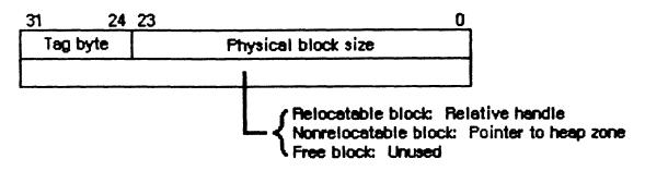
Figure 10. Block Header
