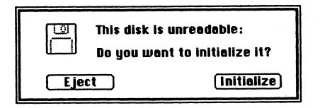
Figure D-1. Disk Initialization Dialog for IOErr
