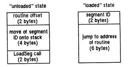
Figure 4. Format of a Jump Table Entry
