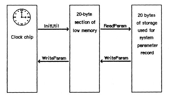
Figure 7. Function of Parameter RAM Utilities
