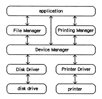
Figure 1. Communication with Devices
