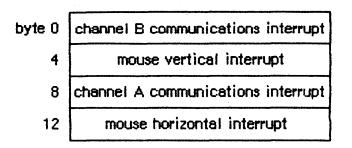
Figure 9. Level-2 External/Status Interrupt Vector Table
