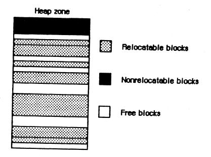
Figure 1. A Fragmented Heap
