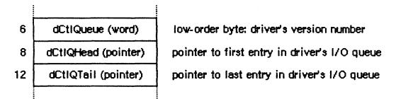
Figure 5. Driver I/O Queue Structure
