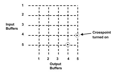
When data enters an input port, an integrated circuit microprocessor turns on the crosspoint of both input and output ports and turns off all other crosspoints for those ports. The only way for the data to travel is to be transmitted through the crosspoint to the correct destination.
