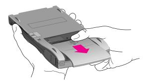
3 Install four AA batteries in the battery compartment. Make sure you position each battery's + and - terminals according to the diagram in the compartment (the batteries don't all have the same orientation). If you install the batteries the wrong way, they may leak and damage your MessagePad. Leaking batteries may be hazardous.
