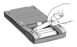
The tab that you pull to remove the batteries should stick out as shown above the topmost battery.
