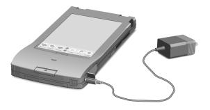
An optional rechargeable battery pack is also available. When the optional battery pack is installed and the power adapter is plugged in, the battery pack recharges.
