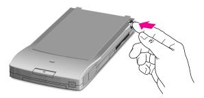
**6** Open the screen lid by pressing in (not down) on the latch at the bottom of the MessagePad and lifting the lid.
