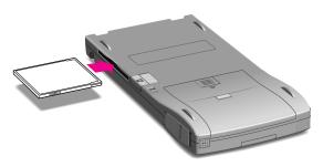
**5** Push the card all the way in to make sure it's connected properly, then lock the card in the slot by pushing up the locking tab.
