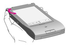
*Optional:* If you purchased the MessagePad power adapter, you can connect it to your MessagePad and plug it in to conserve battery power. The power adapter plugs into the port beneath the rubber flap marked with the --- icon.
