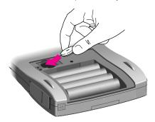
**7** Put back the plate that keeps the backup battery in place. Insert its right end into the slot before you lower the left end (the end with the screw).
