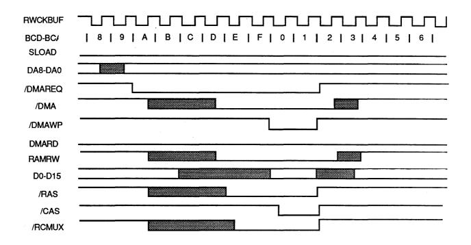
Figure 2.8 DMA write cycle
