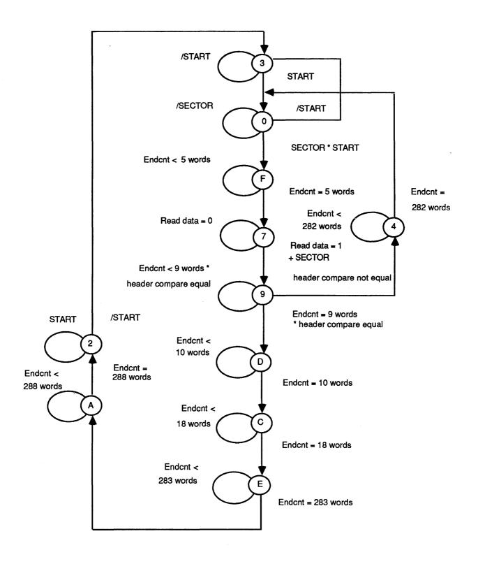
Figure 2.4 Write state sequence
