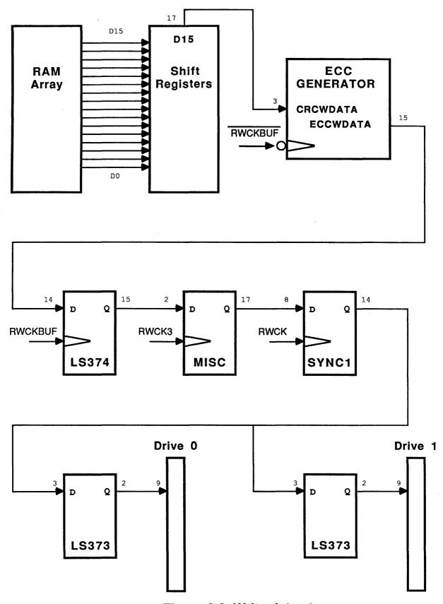
Figure 2.2 Write data stream
