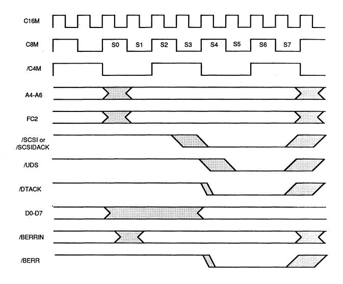
Figure 1.17 SCSI write cycle
