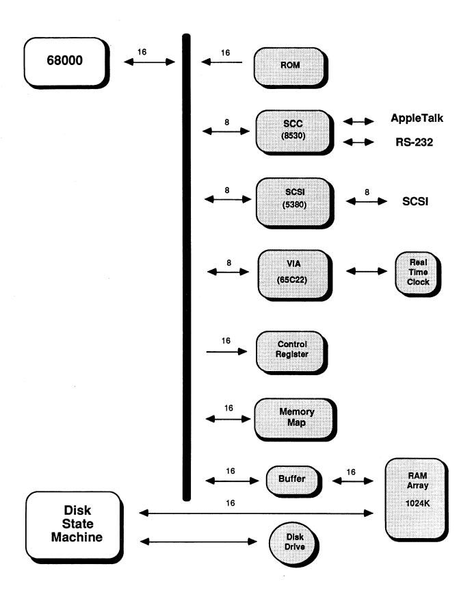
Figure 1.2 Data Bus Block Diagram
