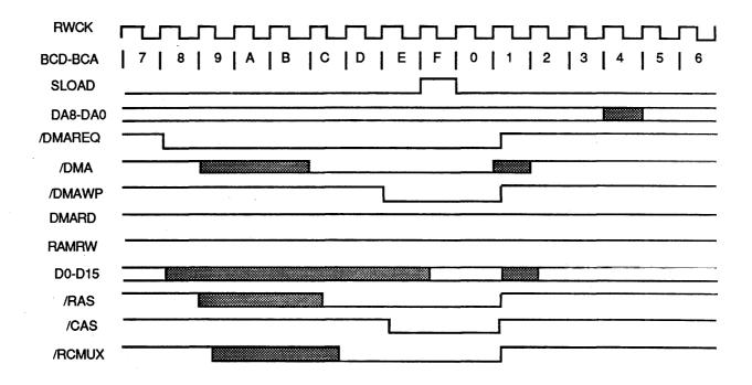
Figure 2.7 DMA read cycle
