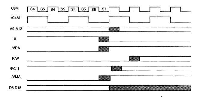
Figure 1.15 VIA write cycle (Best case)
