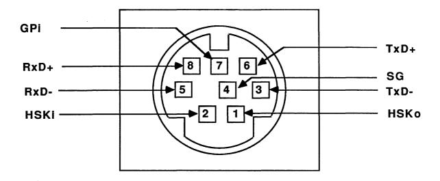
Figure 4.1 MINI DIN-8 connector
