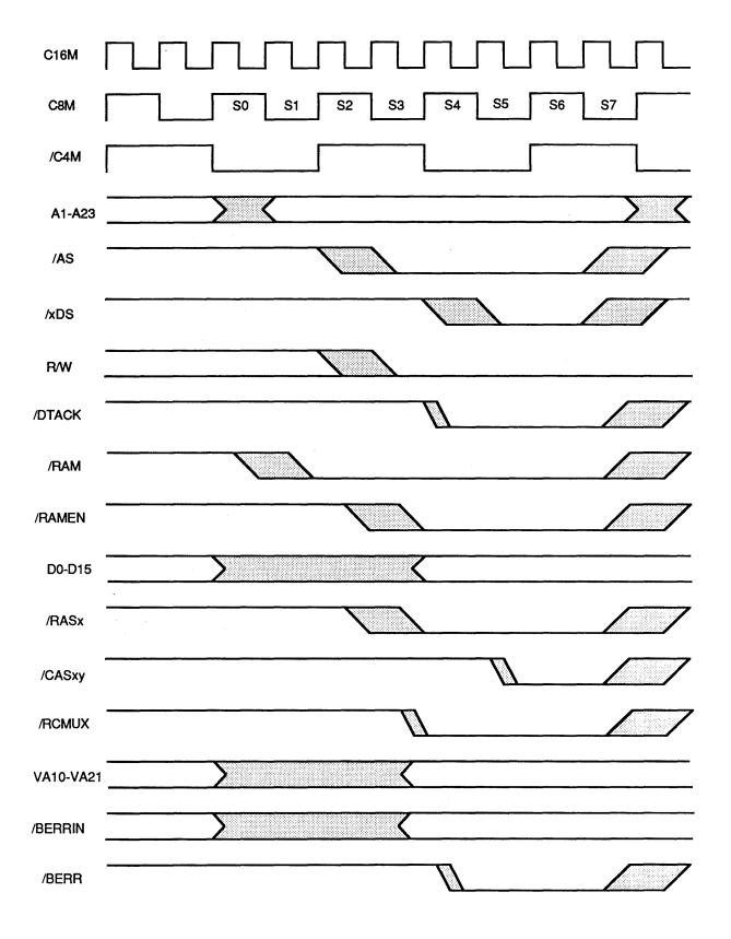
Figure 1.9 RAM write cycle
