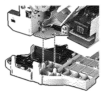
**Replacement Note:** Make sure the bottom cover circular tabs fit into the proper position in the printer frame.
