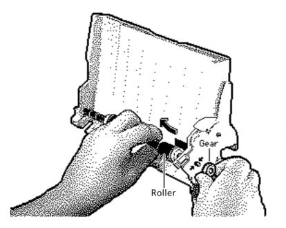
**Caution:** When the roller is removed, the feeder gear is loose. Remove the roller slowly so that the gear will not fly off.
