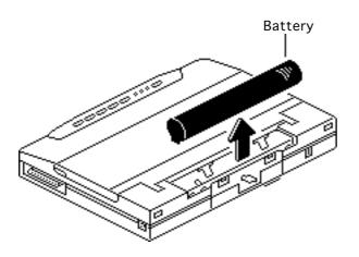
Grasp one end of the battery and remove the battery from the printer.
