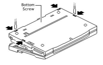
Release the four latches and remove the bottom case.
