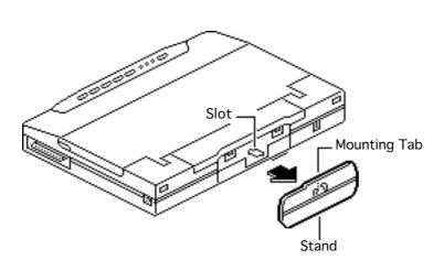
Turn the stand until the mounting tab clears the slot and remove the stand.
