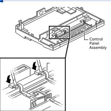
4 Using a small flat-blade screwdriver, release the latches and remove the control panel assembly.
