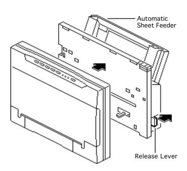
Press the two release levers and remove the automatic sheet feeder.
