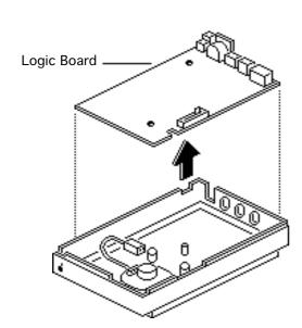
5 Lift the logic board out of the bottom case.
