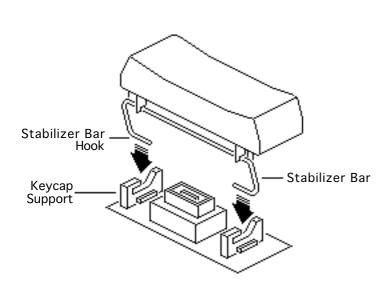
Replacement Note: The Spacebar, Delete, Return, Tab, Shift, Enter, and "0" keys use stabilizer bars to secure the keycaps.
