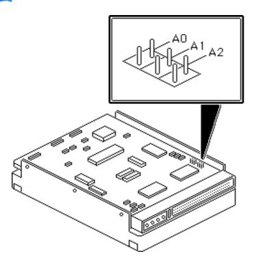
2 Place jumpers on the pairs of pins as shown in the table below.
