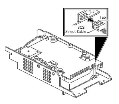
**Important:** You must connect the customer's SCSI select cable to six unkeyed pins on the controller board. Be aware that SCSI select cable connectors differ among drives in both design and location.
