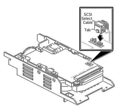
Face the tab up and attach the SCSI cable connector.
