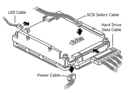
Each drive has four cables that need to be removed before the hard drive is returned. They are
