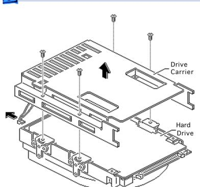
Remove the four screws and lift the carrier from the hard drive.
