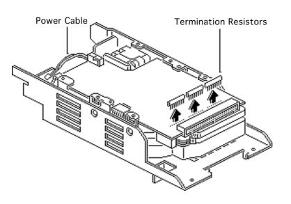
**Note:** The External 20MB SCSI, Rev A replacement hard drive ships prepared for use in external hard drives. You must modify other replacement hard drives for use in external hard drives.
