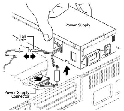
2 Disconnect the power supply connector from the hard drive mechanism.
