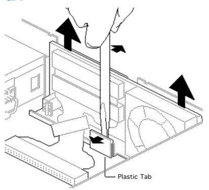
Using a flat-blade screwdriver, push back the plastic tab and lift out the metal fan frame (with fan, HDA-to-case cable, fan cable, and SCSI select switch attached).
